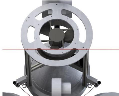
Figure 5.4: Laser alignment procedure for top lamp. When the housing is positioned properly the laser will be able to cross both bolts on the back plate.
