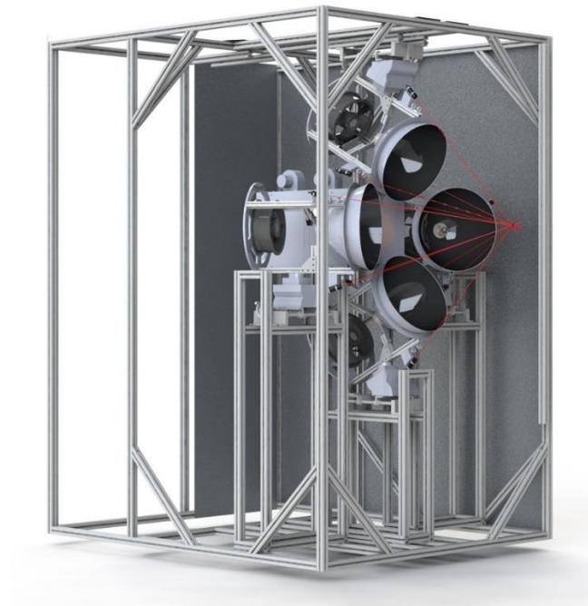
Figure 5.6: laser pointers placed on all 4 metal halide housing for alignment
