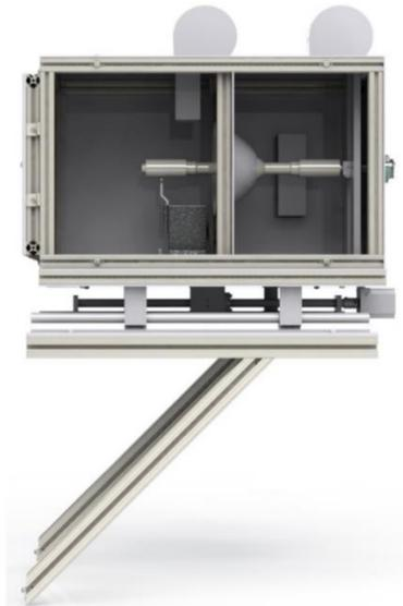
Figure 4.9: Xenon housing placed on pedestal with linear actuator for horizontal translation
