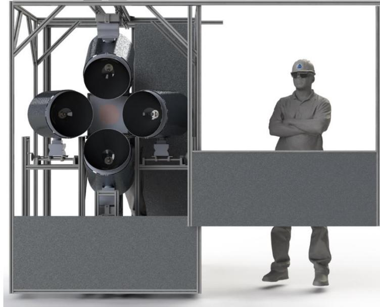
Figure 5.1: Rendering of the 13kW high flux solar simulator
