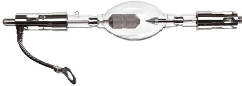
Figure 4.7: Philips LTI 3kW-HS Standard Xenon Lamp with the cathode end on right and anode end on left
