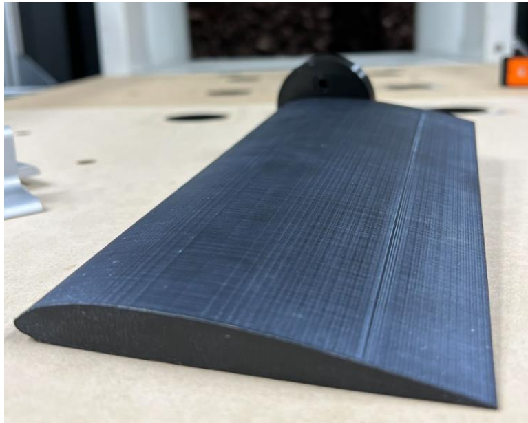
Figure 2-2 3D-Printed Clark Y AR 2 Semispan Wing
