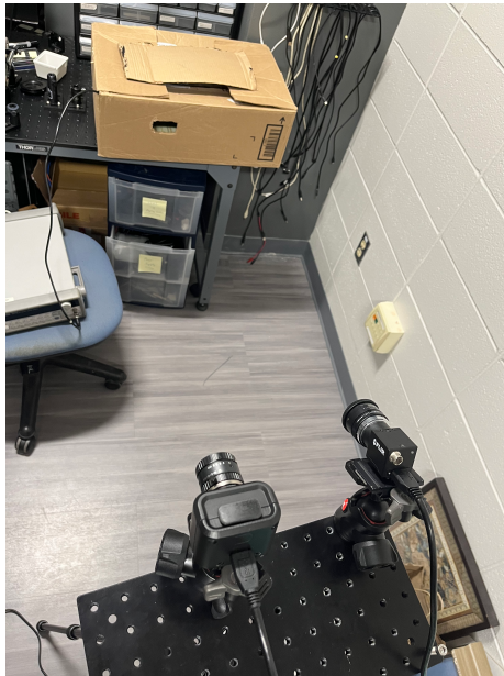
Figure 7.3: Event-based sensor and FLIR camera setup for the calibration experiment.
