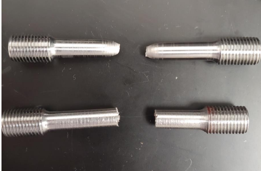
Figure 26: Ductile and Brittle Failure Modes in Unfocused Beam (Top) and Focused Beam (Bottom) As-Built Tensile Bars, Respectively
