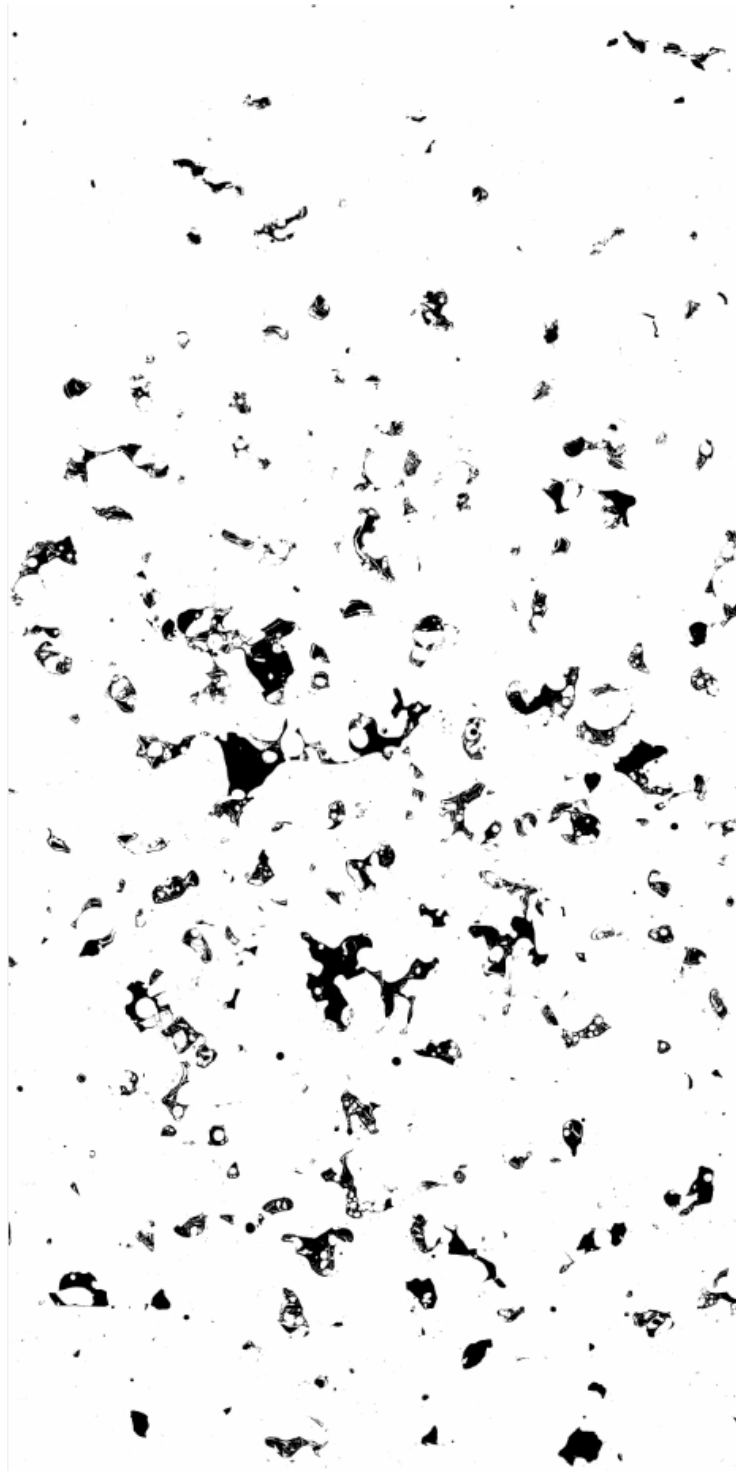
Figure 13: Black and White Porosity Map of Specimen F-2XY
