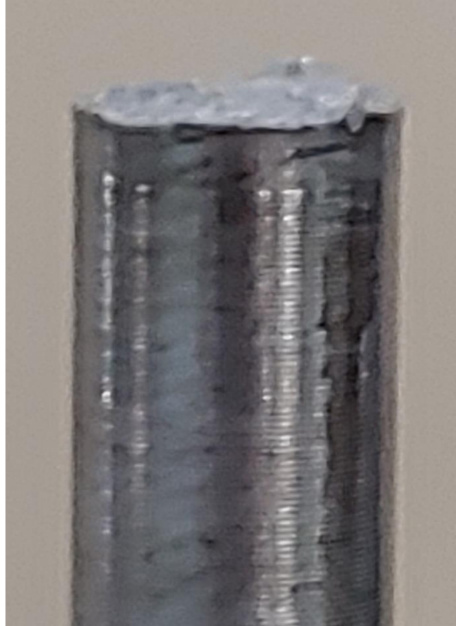
Figure 22: Specimen Failed in Transition Radius
