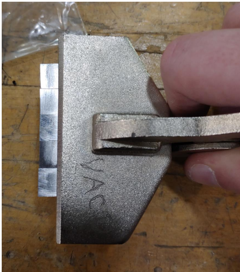
Figure 10: Density Cube Cutting Grip
