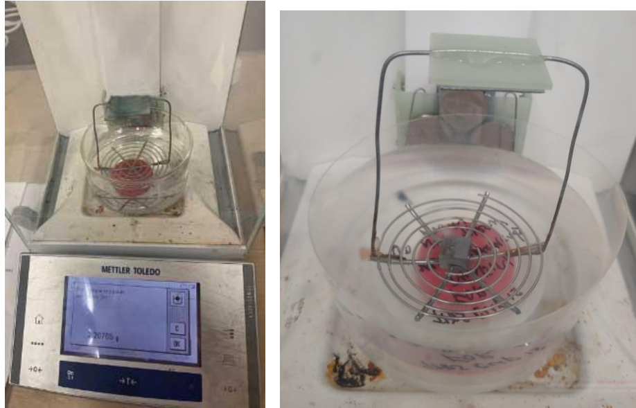
Figure 9: Equipment used for ASTM D790 density measurement: (left) scale with buoyancy fixture, (right) close up of submerged cube being measured for its weight in water
