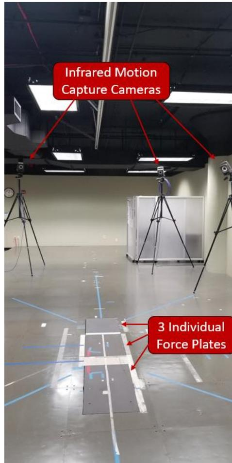
**Figure 3:** Motion capture volume used for data collection in this study. Located in the University of Dayton’s Motion Analysis Lab
