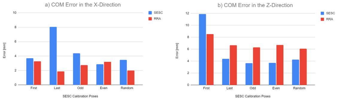
**Figure 4:** COM Error of both the RRA and SESC estimation in the a) x and b) z direction for the PVC humanoid model
