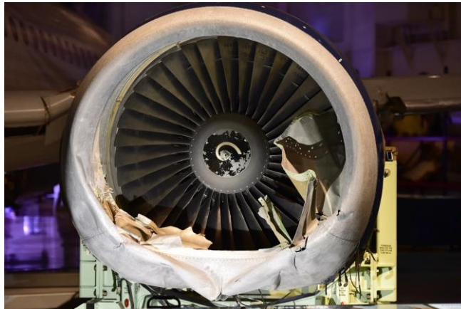
Figure 1: Aftermath of US Airways Flight 1549 Turbine Engine Bird Strike; Photograph provided by AOPA [5]
