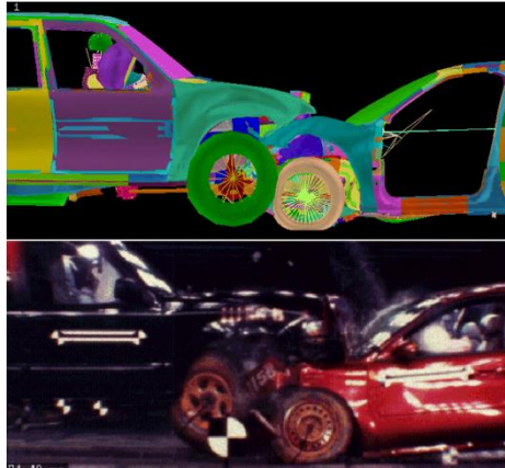
Figure 4: Automotive Crash Simulation (Top) vs. Physical Crash (Bottom); Photo Provided by Ford Motor Company [11]
