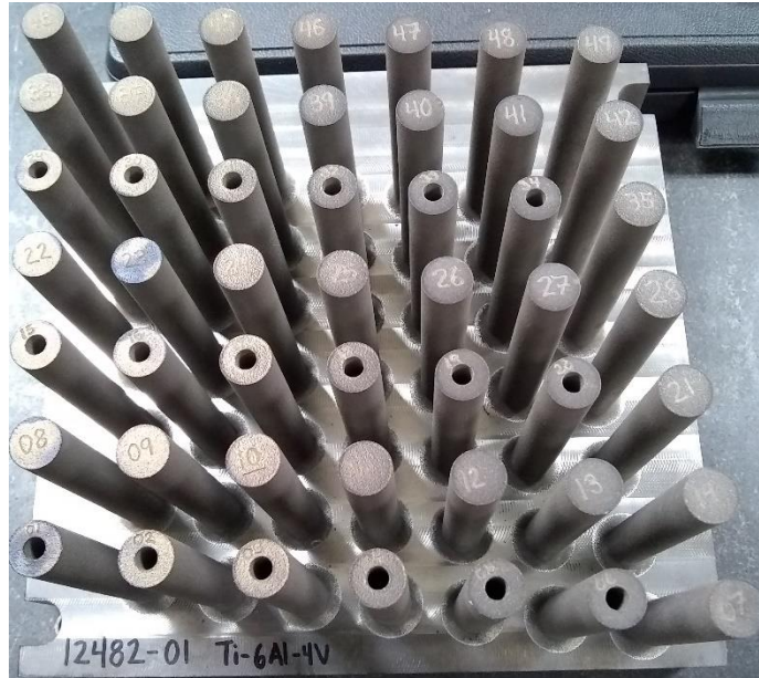
Figure 44: Post AM Build with Specimens Attached to Build Plate
