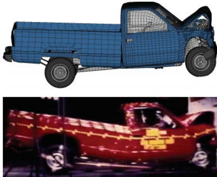
Figure 2: Parallel Simulation (Top) of a Physical Truck Crash (Bottom) [8]
