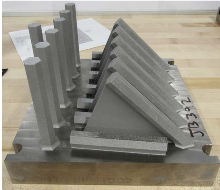
Figure 65: Vertical, Diagonal, and Horizontal AM Ti-6Al-4V Specimens on Build Plate
