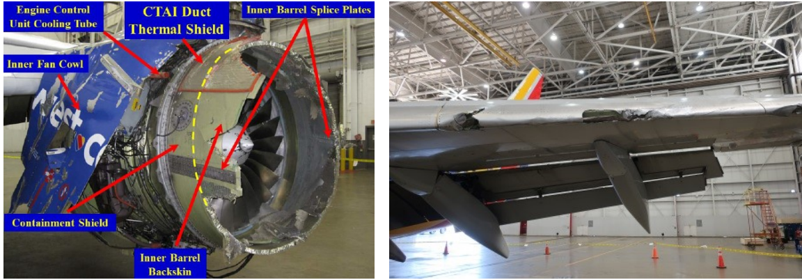
Figure 4: Damage Resulting from Southwest Flight 1380 Engine Failure [12]
