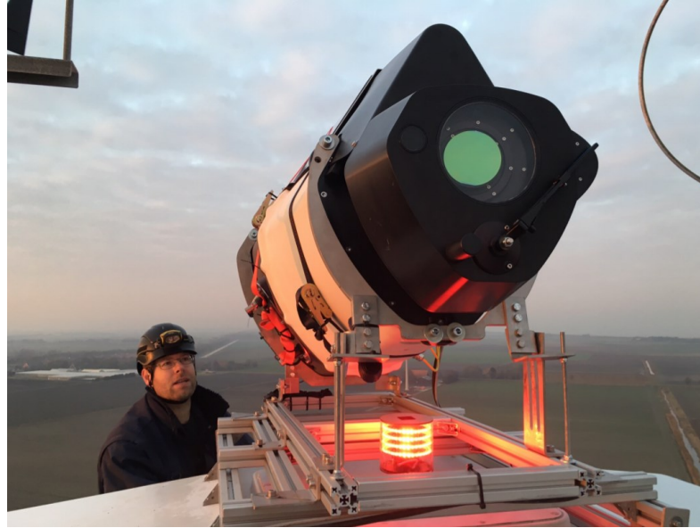
Figure 15. The IRP Wind ScanFlow project used a ZephIR lidar for velocity measurements. [41]
