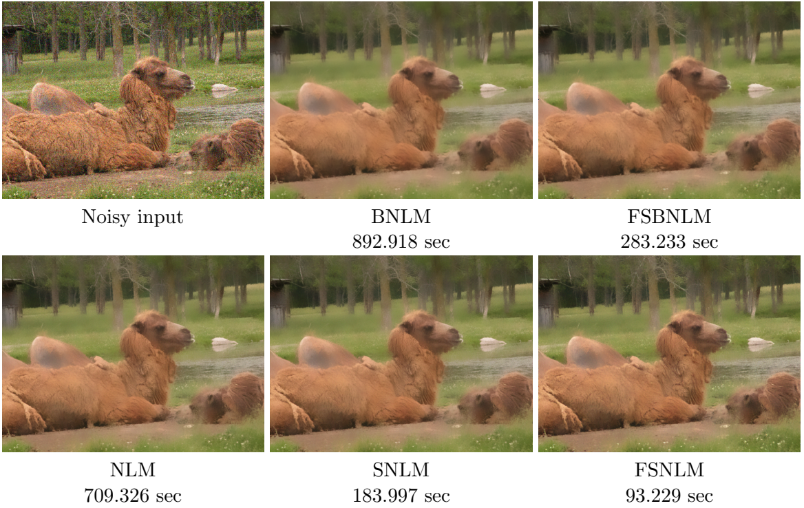
Figure 4.9: Example non-local means and block non-local means results. Parameters used: \sigma = 10 , \theta = 85 , W = 61 , B = 3 . Reported times are obtained to yield an MSE of 5 between naive implementations and fast versions.
