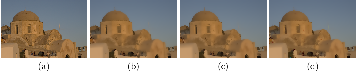
Figure 4.3: Example bilateral filtering results. Parameters were (a-d), \sigma = 10 , \theta = 51 , W = 61 . (a) Input image (b) BF (61.98 sec), (c) BF implementation of [4] (2.96 sec), (d) Quasi-FSBF (0.93 sec). Iteration numbers were chosen to yield PSNR \geq 41.14 dB relative to the BF output. Image from [6].
