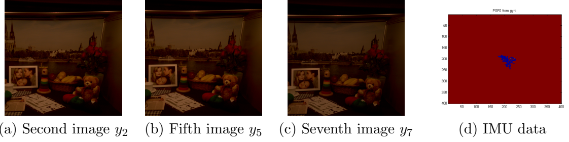
Figure 10.5: Example of recorded IMU \theta_0 and image sensor \{y_1, \dots, y_N\} data in a burst shot mode of N = 12 images.
