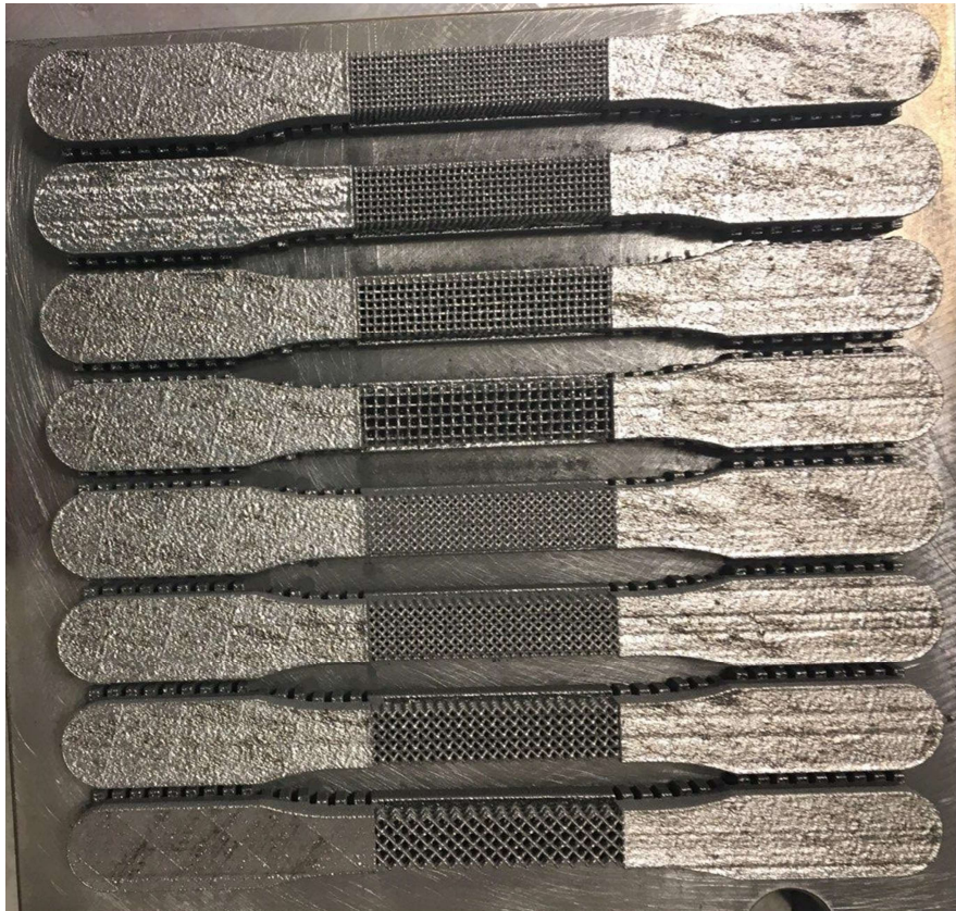
Figure 23. Tensile specimen via SLM, diamond and cubic lattices
