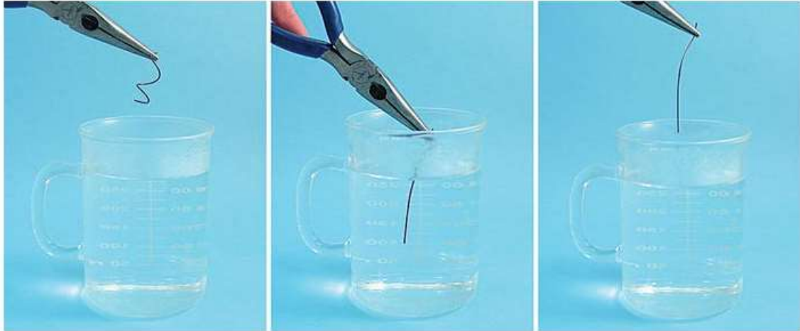
Figure 1. Nitinol shape memory from non-original form to original due to high temperature liquid [40]
