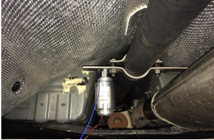
Figure 4.4: Shaker placement on the rear drive shaft
