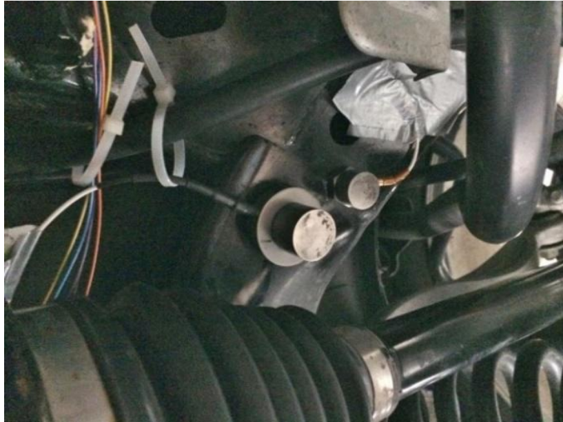
Figure 4.1: One of the two piezoelectric PMAs installed on the rear subframe
