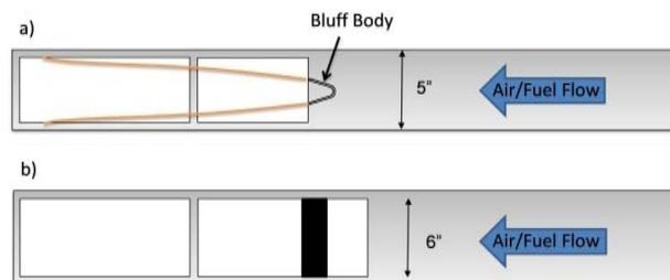
**Figure 5. Schematic of bluff body rig showing optical access: a) top view b) side view**
