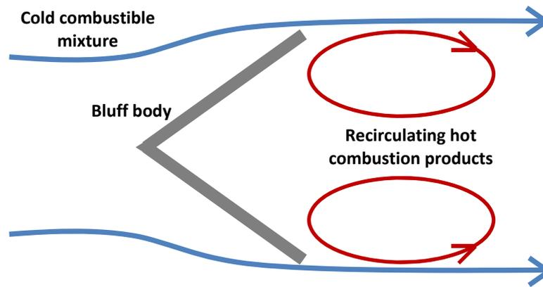
**Figure 1. Schematic of bluff body flame stabilization – Reproduced from Law (2006)**
