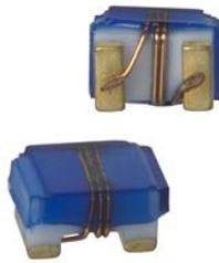
Figure 35. 900 MHz loopstick antenna.
