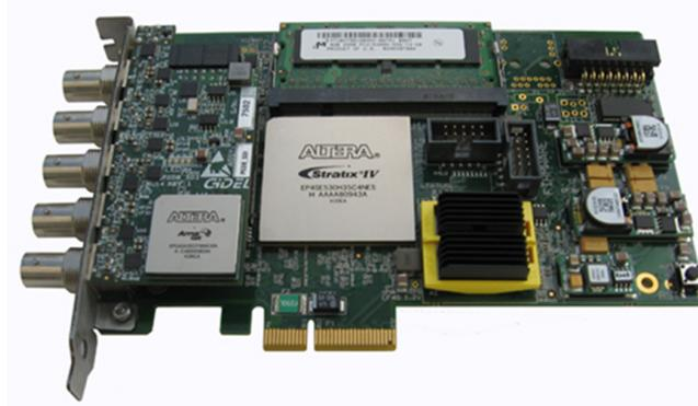
Figure 4.1: PROCeIV FPGA Card from GiDEL
