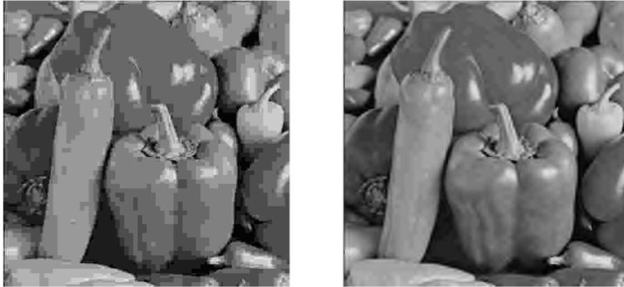
Figure 2.1: Distortion of compressed image at 0.1 bpp using JPEG (left) and JPEG2000 (right)
