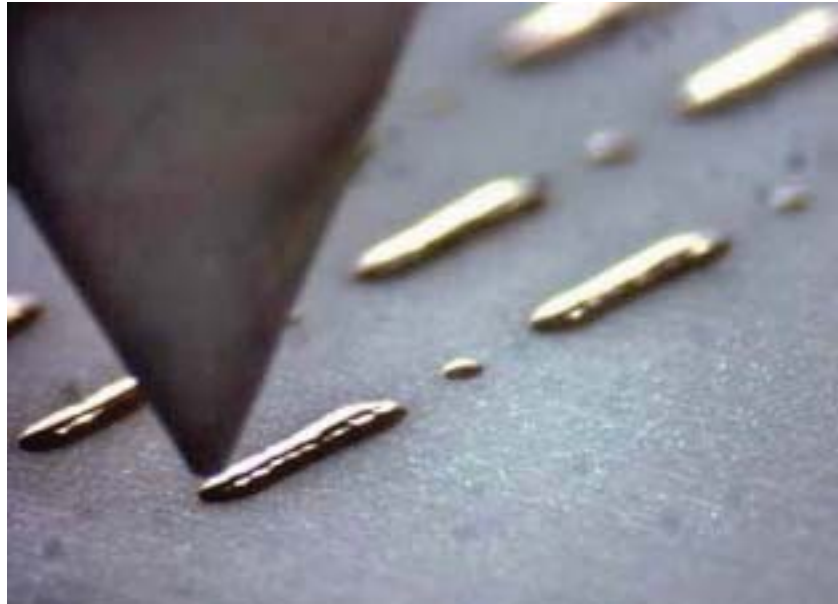
Figure 4.2 Deposition of material with a micro-dispensing nozzle.
