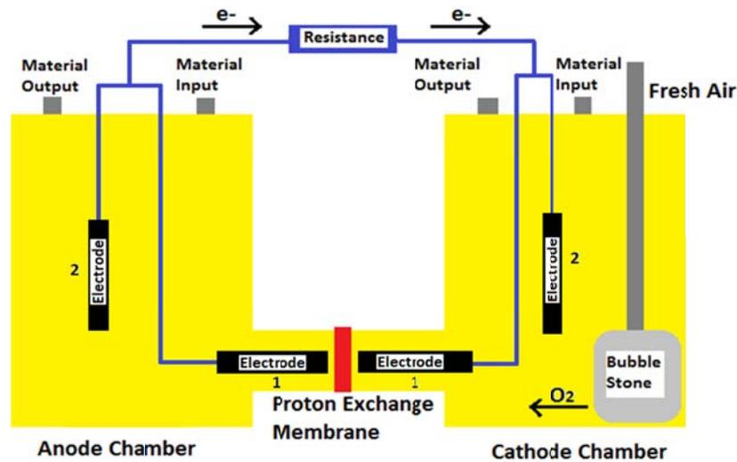
**Figure 4:** Sketch of MFC model with electrodes in different positions. Electrical properties were monitored when the electrode pairs were positioned at matched positions 1 or positions 2.
