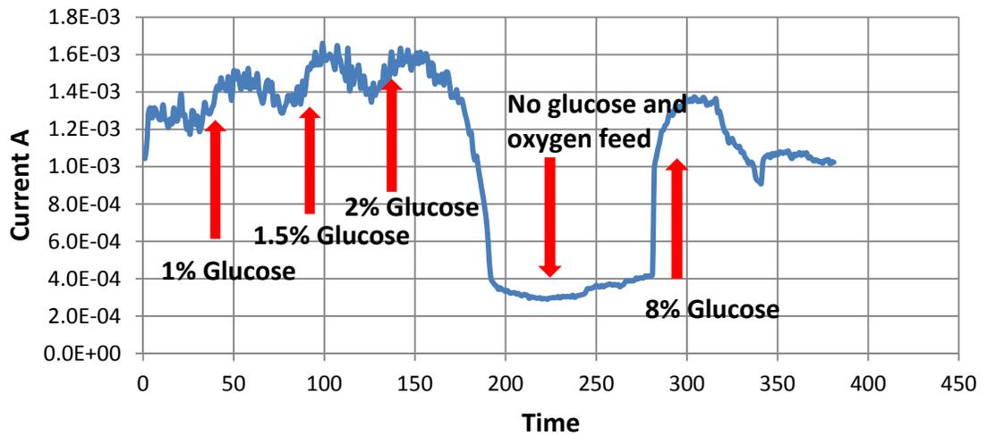
**Figure 6:** Curves of current output relative to time for experiments of varied concentration of glucose in LB medium.
