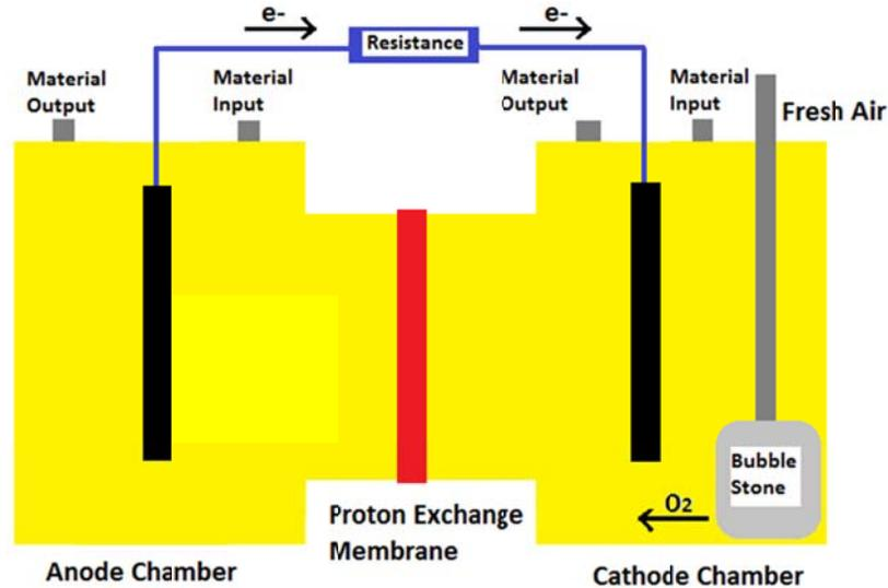
**Figure 3:** Sketch of bottle MFC model. The black rectangles represent electrodes; the red one is proton exchange (Nafion) membrane.
