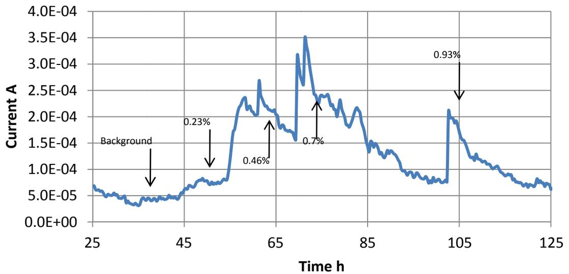
**Figure 8:** Curves of current outputs relative to time for experiments of varied concentration of glucose in MS medium.
