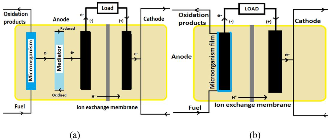
**Figure 2:** Sketch of mediated transfer and biofilm transfer in MFCs.
