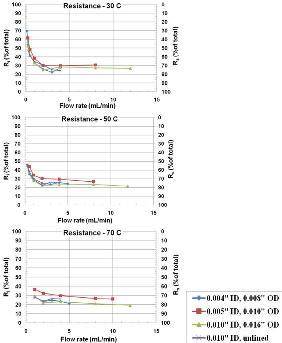
Figure 3-11: Comparing Internal ( $R_i$ ) to Surface ( $R_s$ ) Resistance as a Percentage of Total Resistance for All Tube Sizes and Inlet Temperatures
