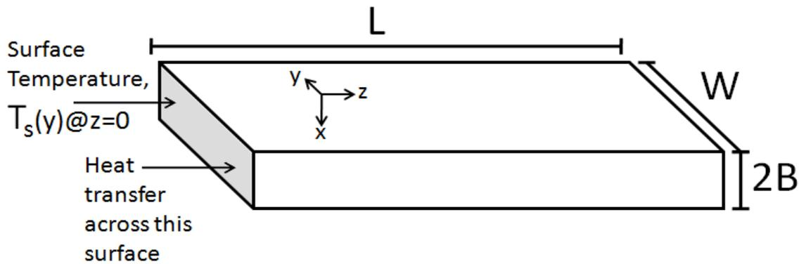
Figure 3-9: Illustration of geometry on which overall surface heat transfer coefficient ( $U_s$ ) is based.
