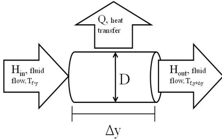
Figure 3-5: Fluid energy balance
