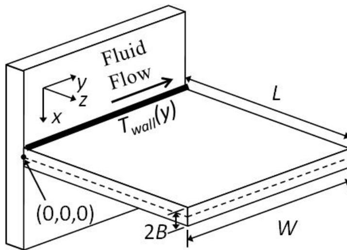
Figure 3-6: Cooling fin geometry
