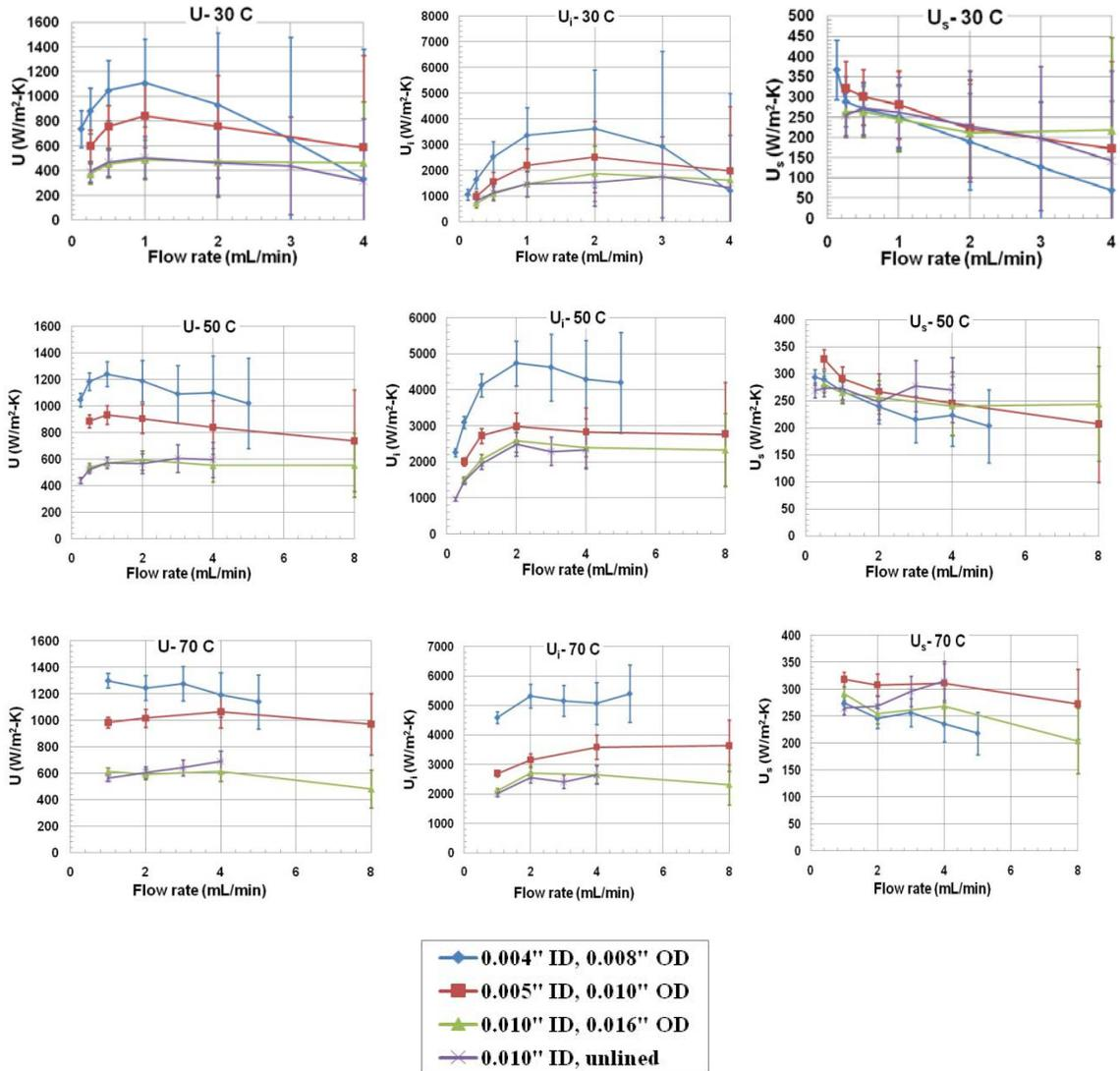
Figure 3-10: Total, internal, and surface heat transfer coefficients ( $U$ ,  $U_i$ ,  $U_s$ ) for all tube sizes and inlet temperatures.
