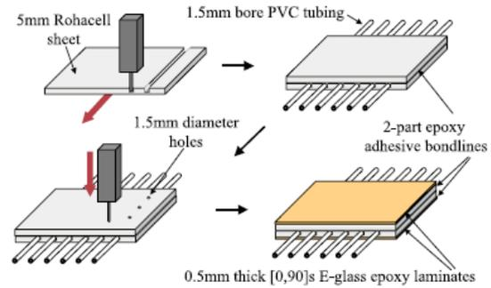
Figure 1-2. Manufacture of vascular sandwich panels [10]
