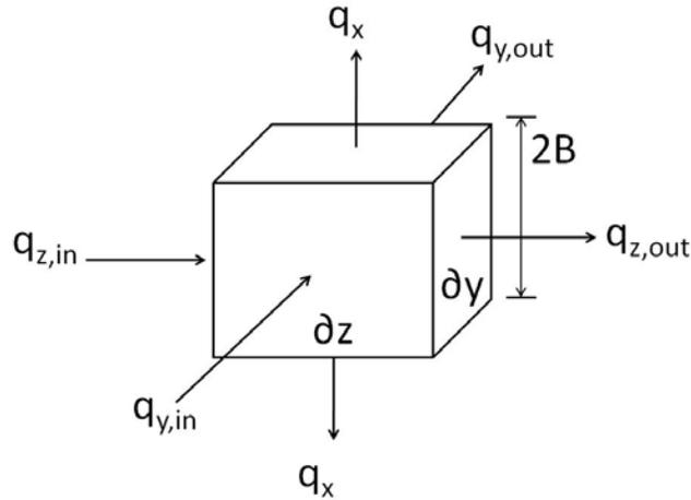
Figure 3-7: Cooling fin energy balance
