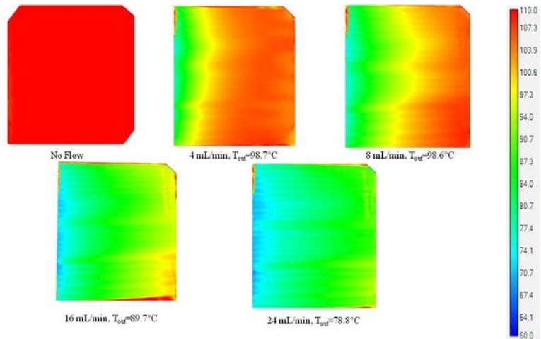
Figure 3-3: Thermal images for various flow rates. Inlet temperature is 40 °C and oven temperature is 110 °C.
