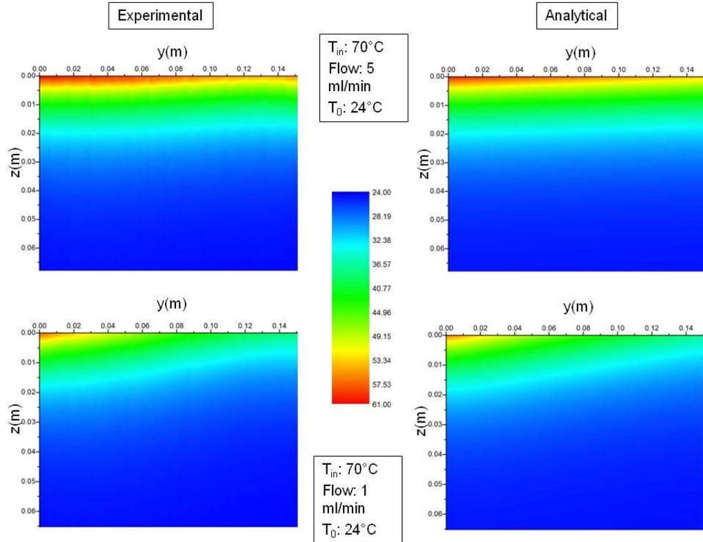
Figure 3-8: 2D temperature profile comparison of experimental thermal images to analytical fit
