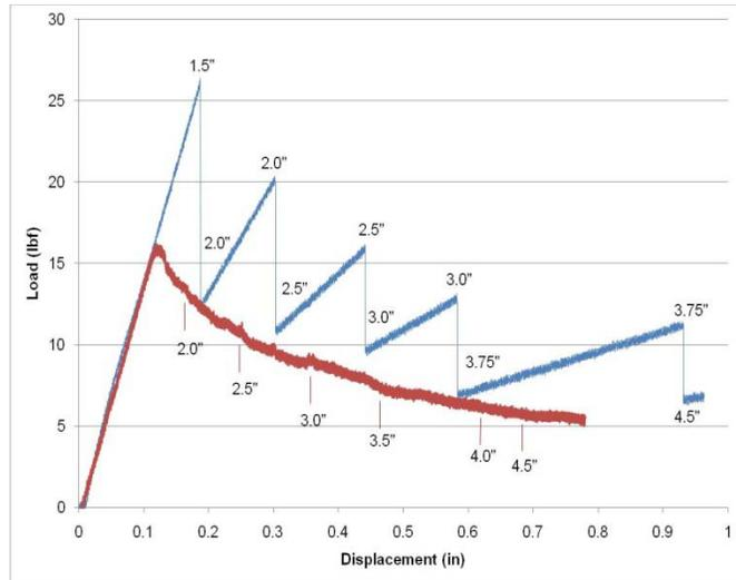
Figure 3-1: Mode I test data comparing the control sample (in red) to a test sample (in blue)
