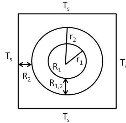
Figure 3-12: Internal heat transfer resistances in series
