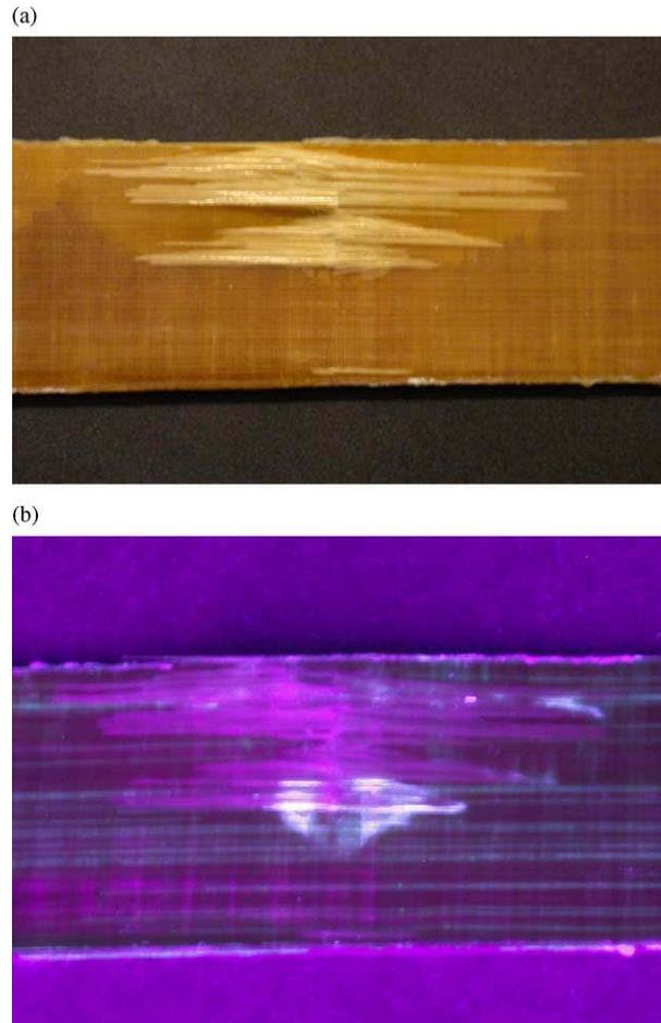
Figure 1-1: Comparison of traditional damage image(a) to ultraviolet illuminated damage(b).[3]
