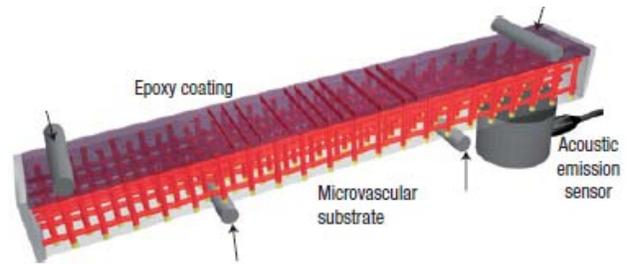
Figure 1-3. 3D microvascular network [12]
