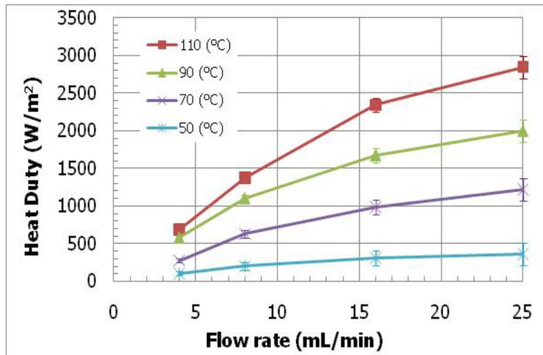
Figure 3-4: Heat duty as a function of flow rate and oven temperature for the multiple tube panel. Inlet temperature is 40 °C
