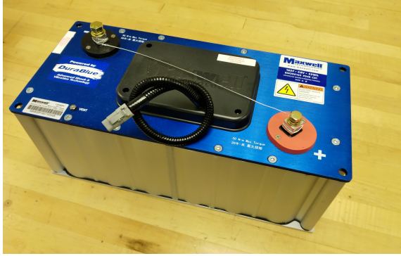
Figure 2: Maxwell ultracapacitor (165 farad-48 volt). Control, Robotics and Mechatronics Laboratory (CRML), Cleveland State University.
