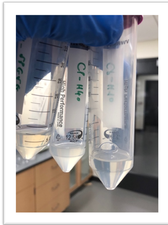
Figure 19. Samples of CP-VPGVG, CP-H10, and CP-H40 were heated up to 60°C which results in clear, semi-turbid, and turbid solutions respectively. Ammonium sulfate was added to CP-VPGVG and CP-H10 to reach the final concentration of 2 M and 1 M individually and salt out the proteins of interest
