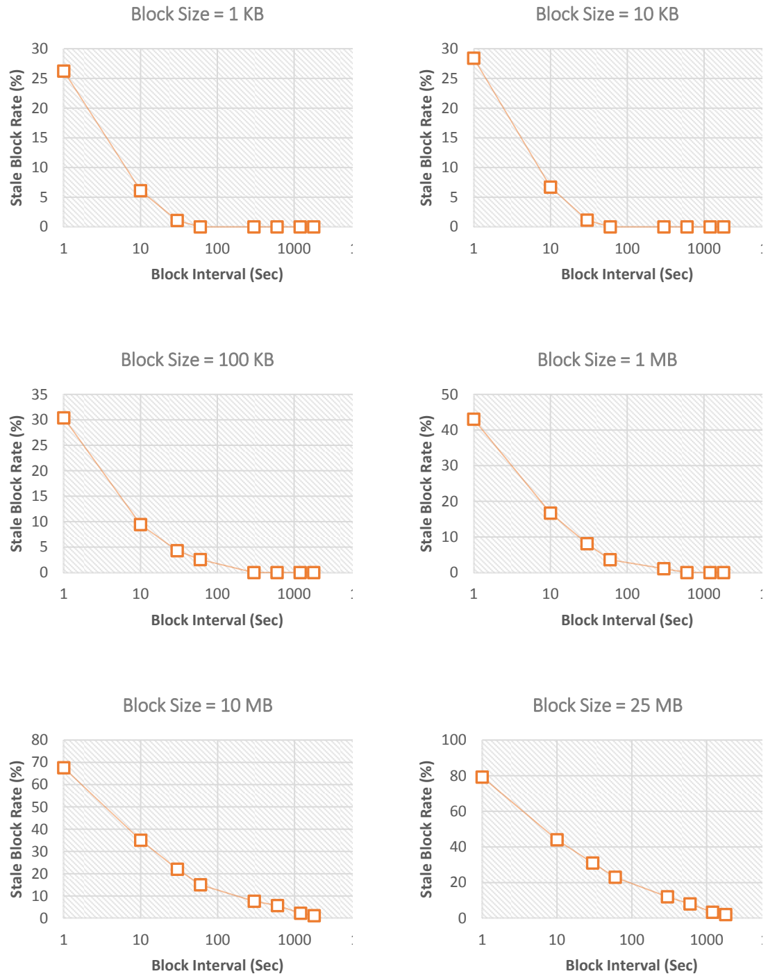
Figure 4-2. Stale block rate as a function of block interval for various block sizes: 1 KB, 10 KB, 100 KB, 1 MB, 10 MB, and 25 MB.
