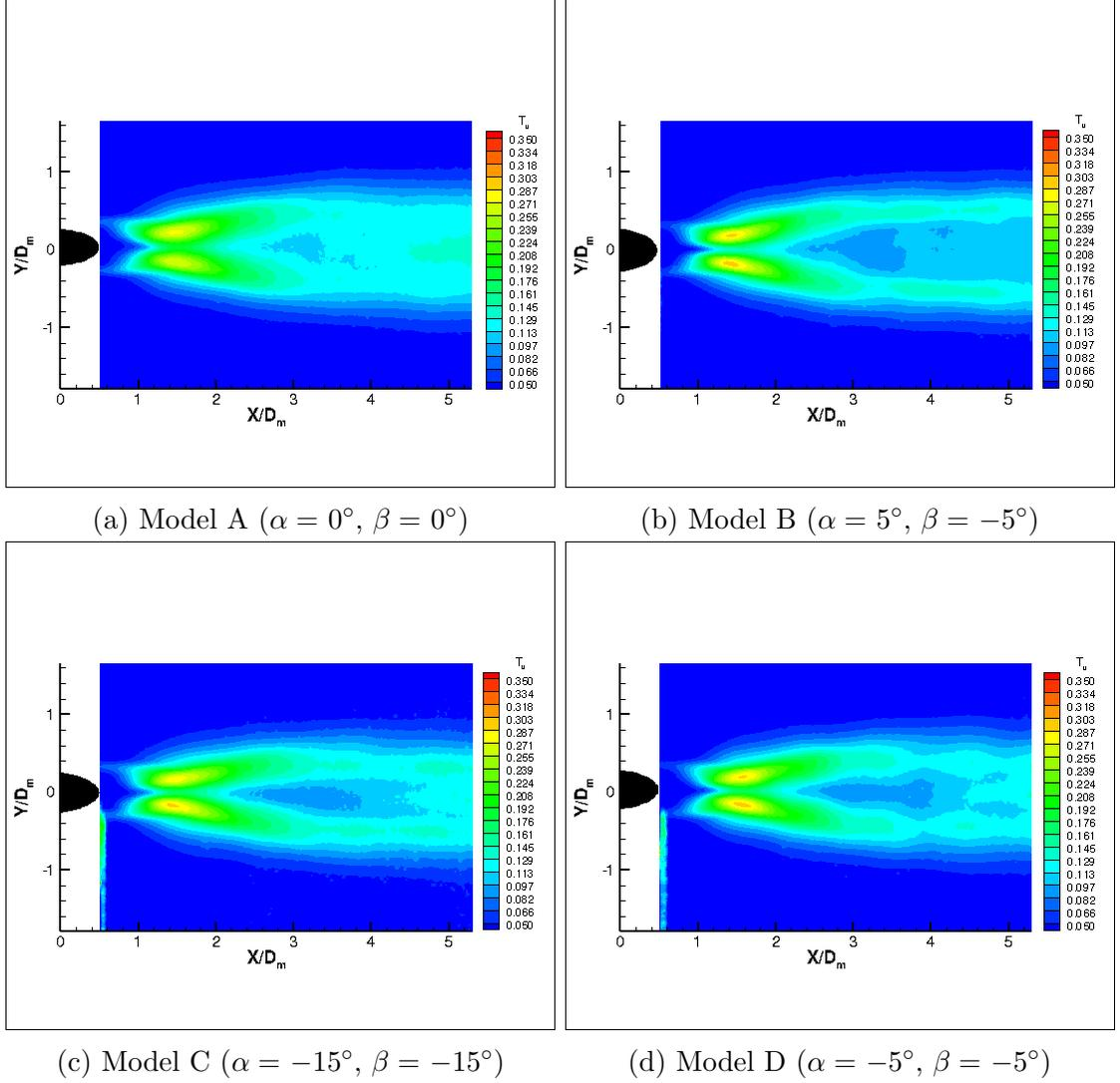
Figure 40: Turbulence intensity of  $u$  fields in the wake of whisker models A-D (Peak cross section  $x$ - $y$  plane)
