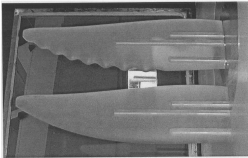
Figure 2: Wind tunnel test articles studying the effect of tubercles observed on humpback whales flippers [49]
