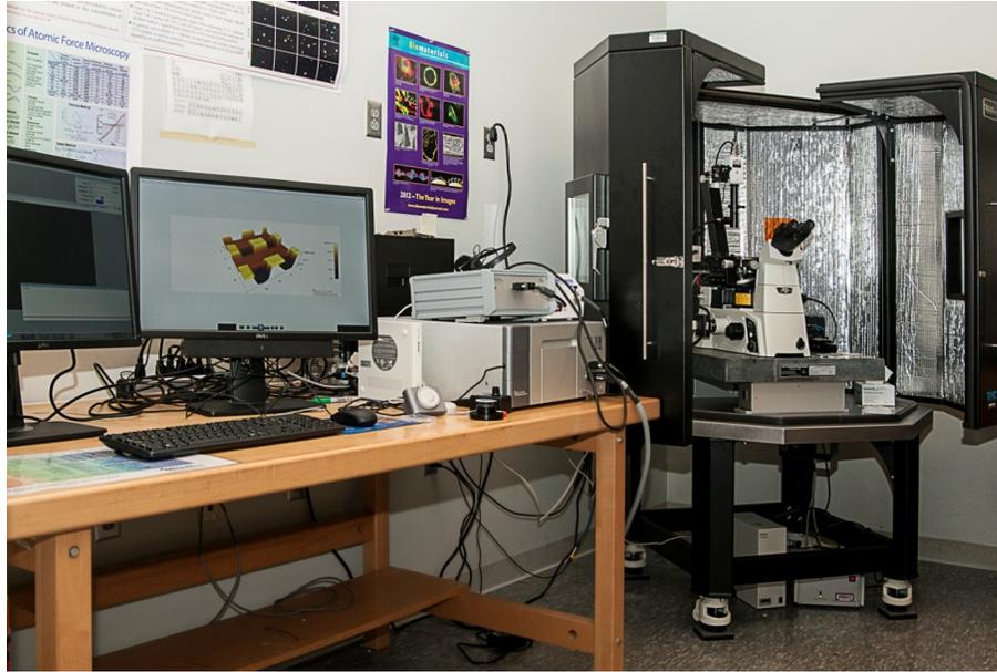
Figure 8: Asylum MFP-3D-IO Atomic Force Microscope at Cleveland State University
