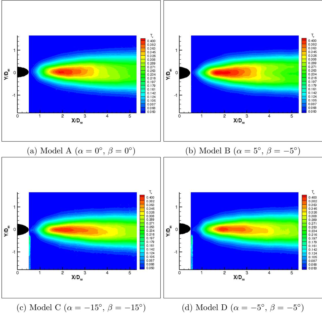
Figure 41: Turbulence intensity of  $v$  fields in the wake of whisker models A-D (Peak cross section  $x$ - $y$  plane)
