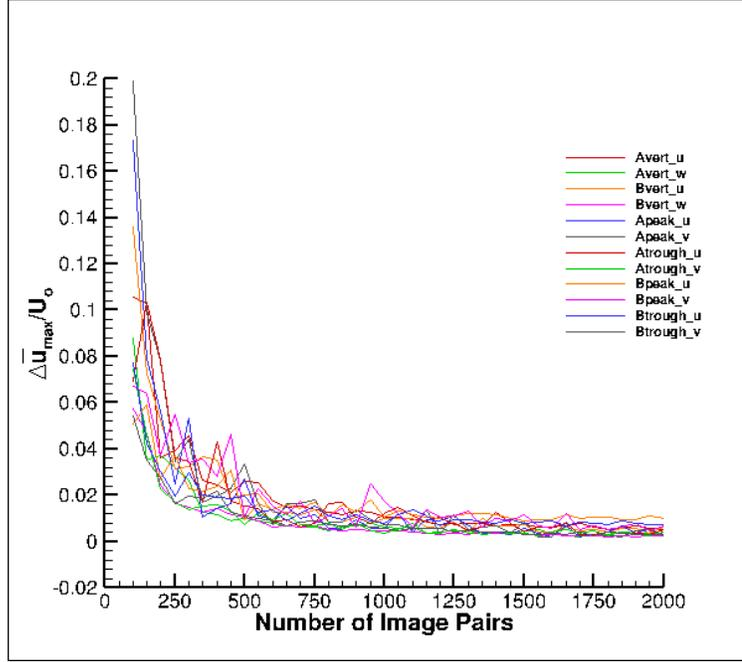
Figure 29: Convergence of ensemble averaged velocity fields in vertical centerline, peak and trough measurement planes
