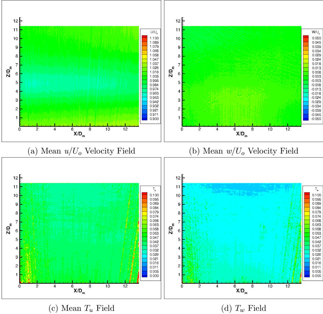
Figure 26: Water channel flow characterization: velocity and turbulence fields in the vertical centerline plane ( $x$ - $z$ )
