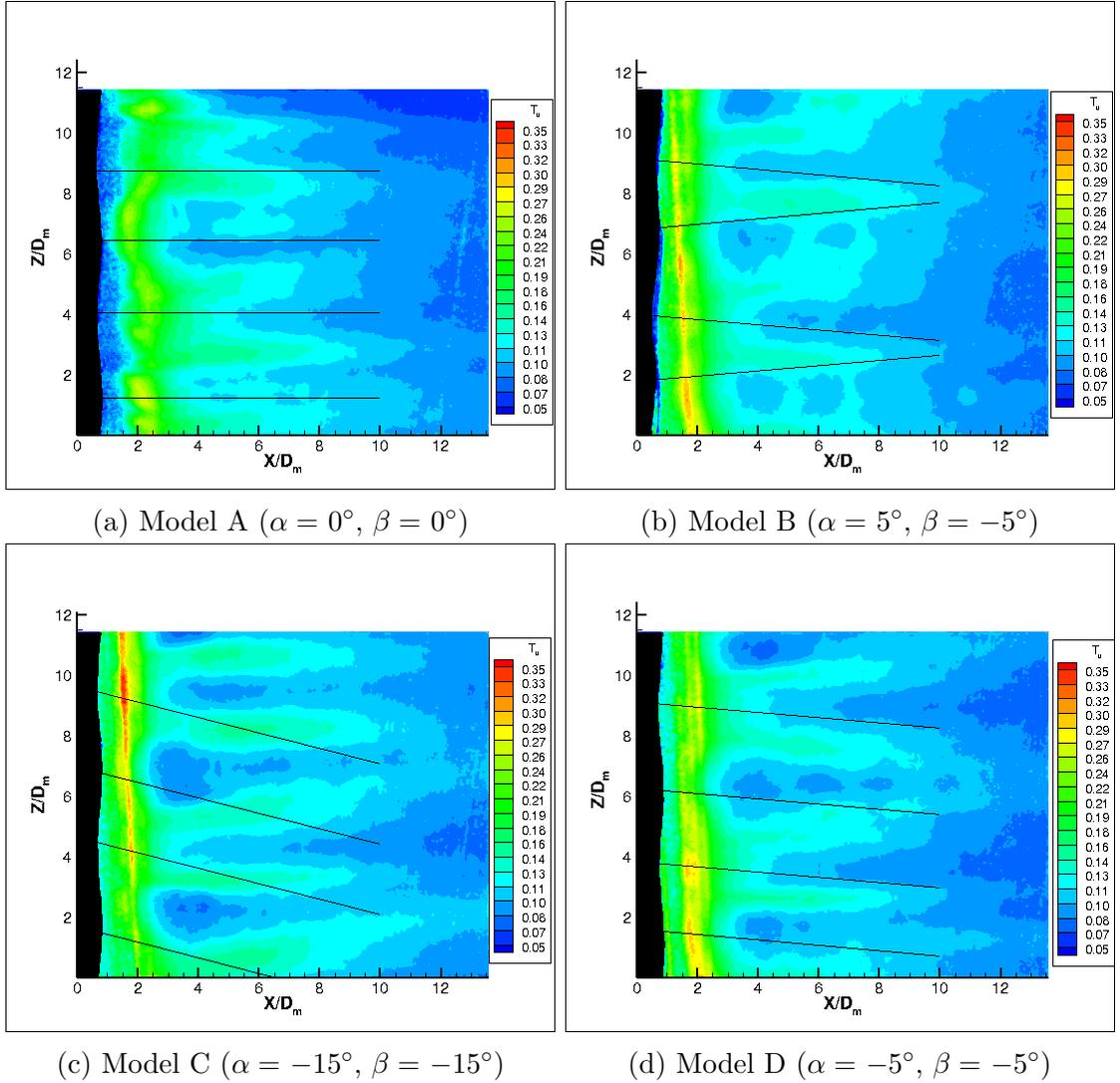
Figure 34: Turbulence intensity of  $u$  fields in the wake of whisker models A-D (Vertical center  $x$ - $z$  plane)
