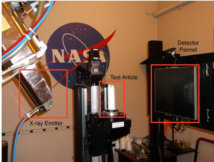
Figure 9: CT Scanner at NASA Glenn Research Center
