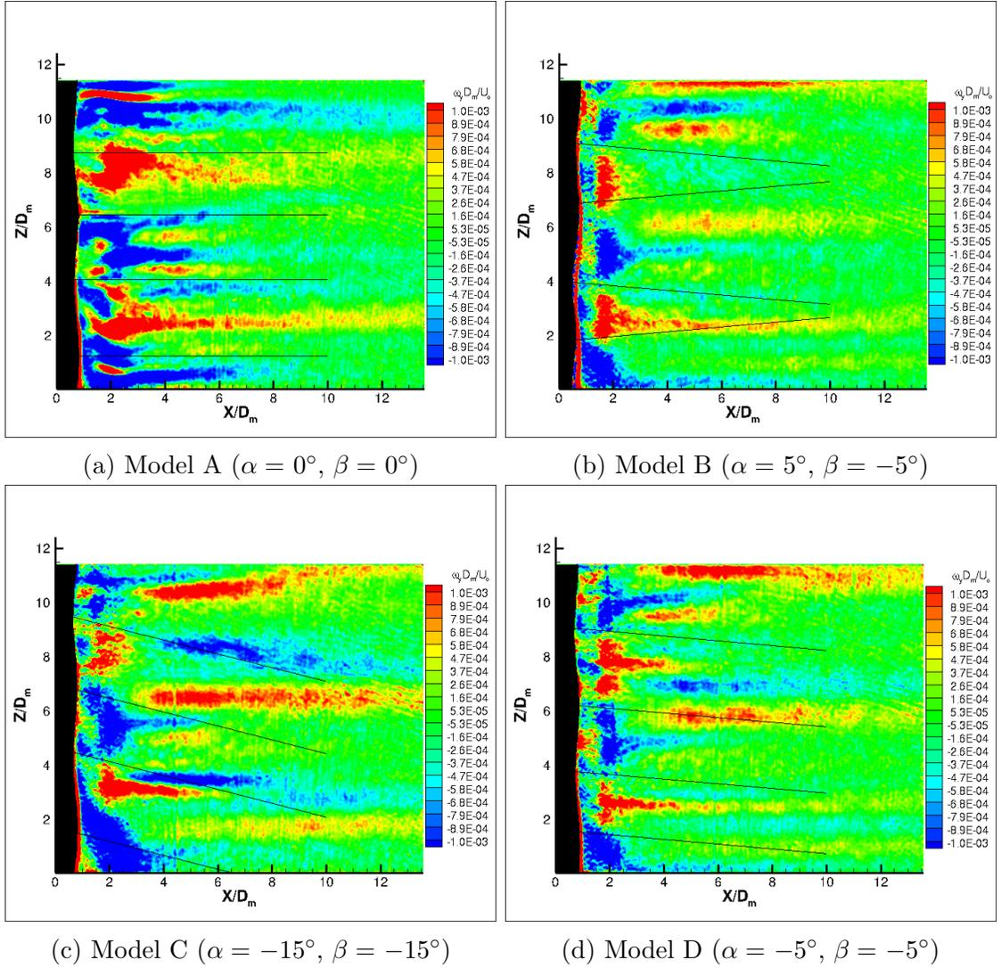
Figure 33: Normalized  $\omega_y$  vorticity fields in the wake of whisker models A-D (Vertical center  $x$ - $z$  plane)
