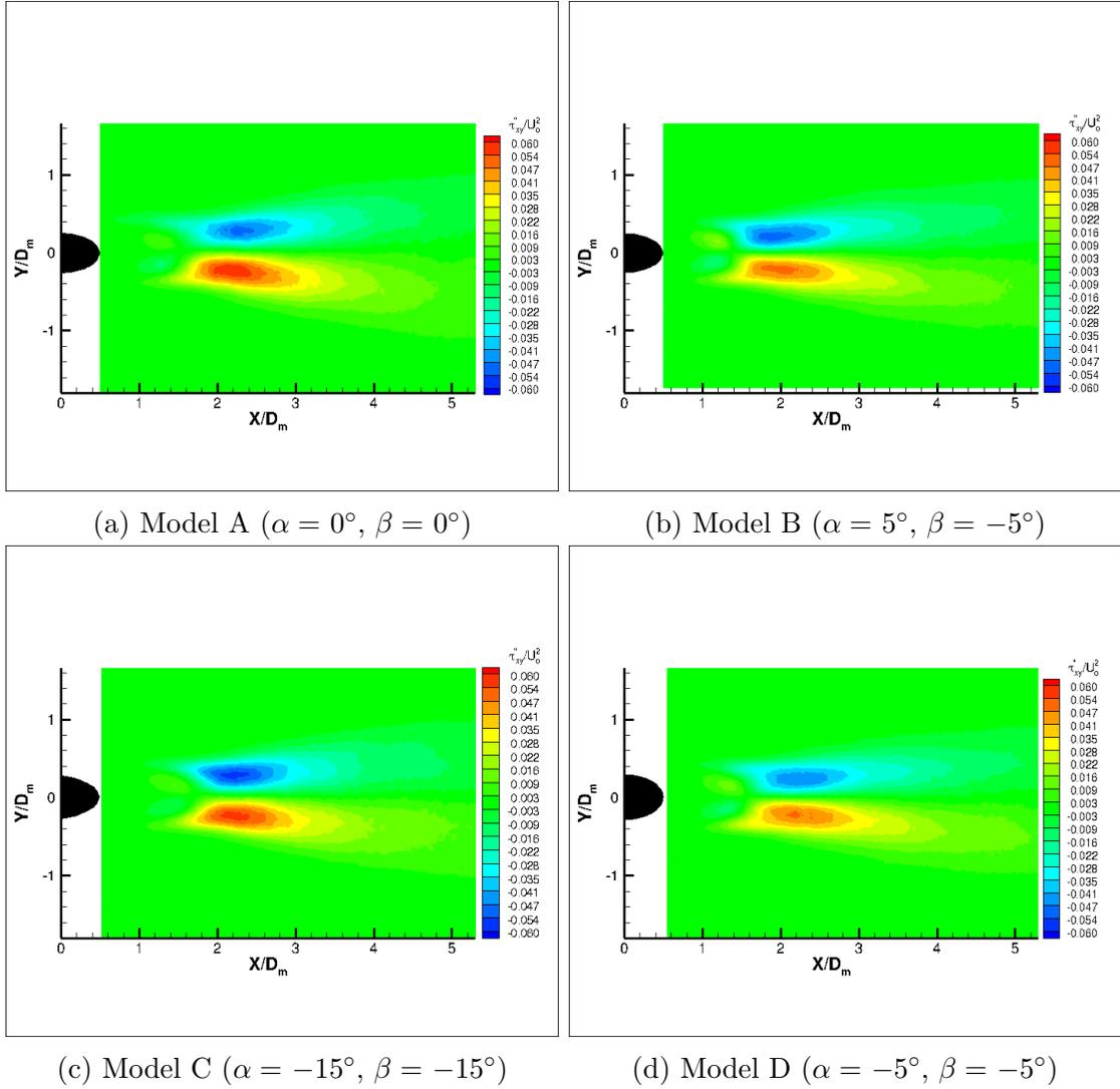
Figure 48: Reynolds shear stress fields in the wake of whisker models A-D (Trough cross section  $x$ - $y$  plane)
