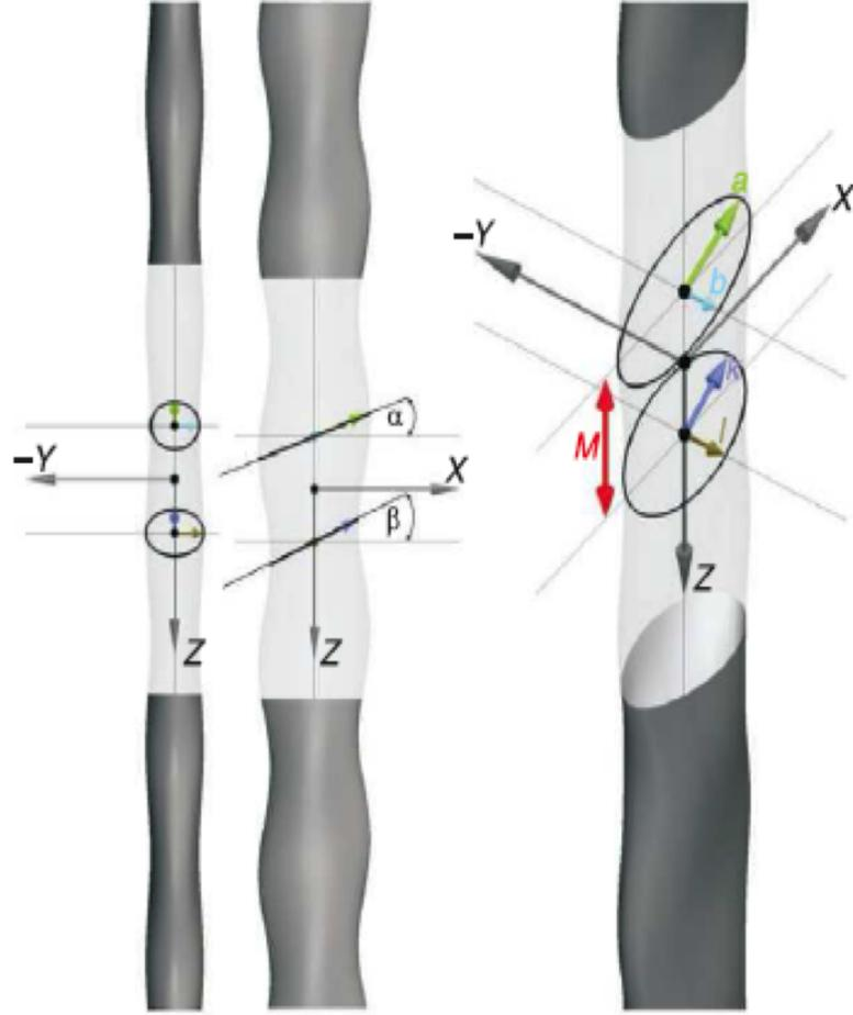
Figure 6: 7 Parameter Whisker Definition provided by Hanke et al. [29]
