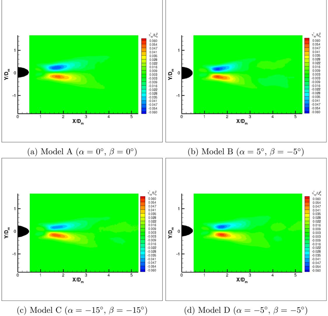
Figure 42: Reynolds shear stress fields in the wake of whisker models A-D (Peak cross section  $x$ - $y$  plane)
