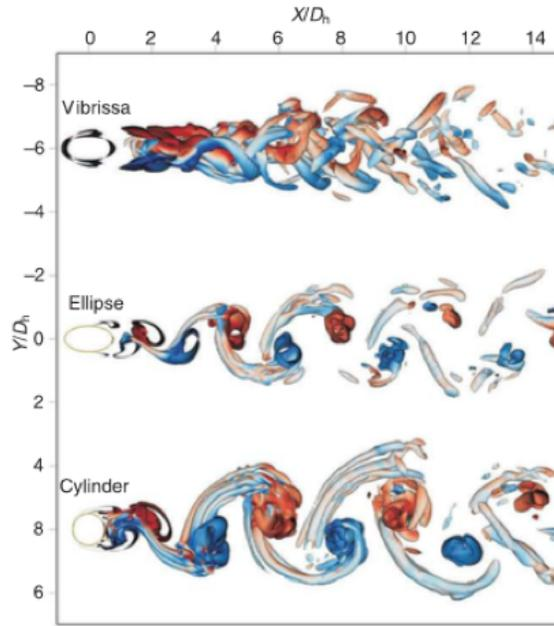
Figure 5: Comparison of wake Q-criterion (rotational strength) of circular, elliptical, and whisker-like cylinders. Showing the whisker’s ability to break coherent vortex structures [29]
