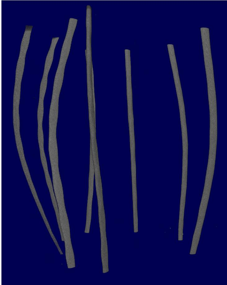
Figure 11: Whisker Reconstruction from CT Scanner
