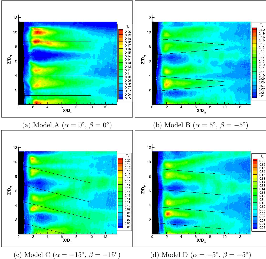
Figure 35: Turbulence intensity of  $w$  fields in the wake of whisker models A-D (Vertical center  $x$ - $z$  plane)
