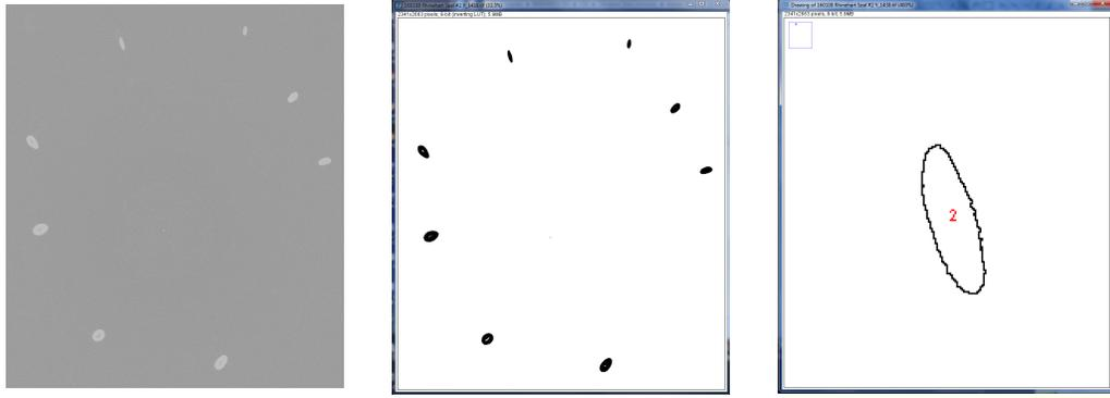
(a) Whisker Cross Section Image from CT Scanner (b) Results of ImageJ Threshold Analysis (c) Results of ImageJ Particle Analysis
