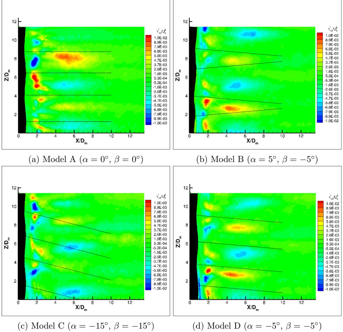
Figure 36: Reynolds shear stress fields in the wake of whisker models A-D (Vertical center  $x$ - $z$  plane)
