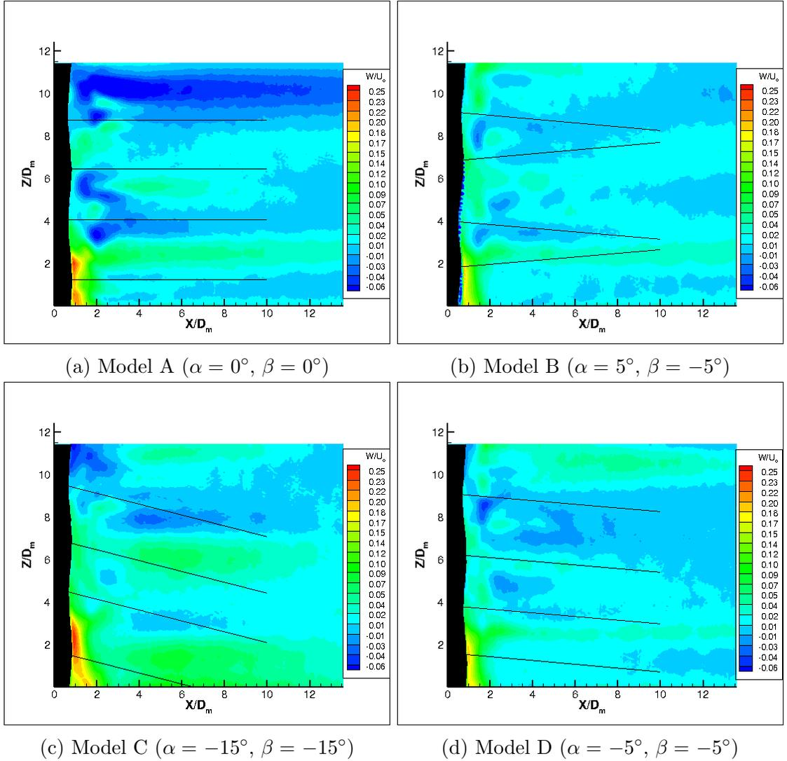
Figure 32: Normalized mean  $w$  velocity fields in the wake of whisker models A-D (Vertical center  $x$ - $z$  plane)
