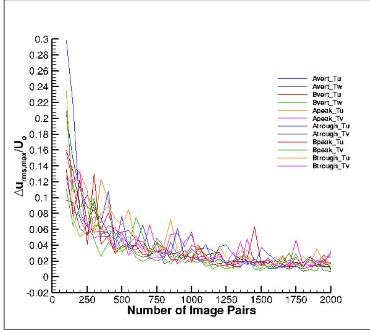
Figure 30: Convergence of ensemble averaged root-mean-square velocity fields in the vertical centerline, peak and trough measurement planes
