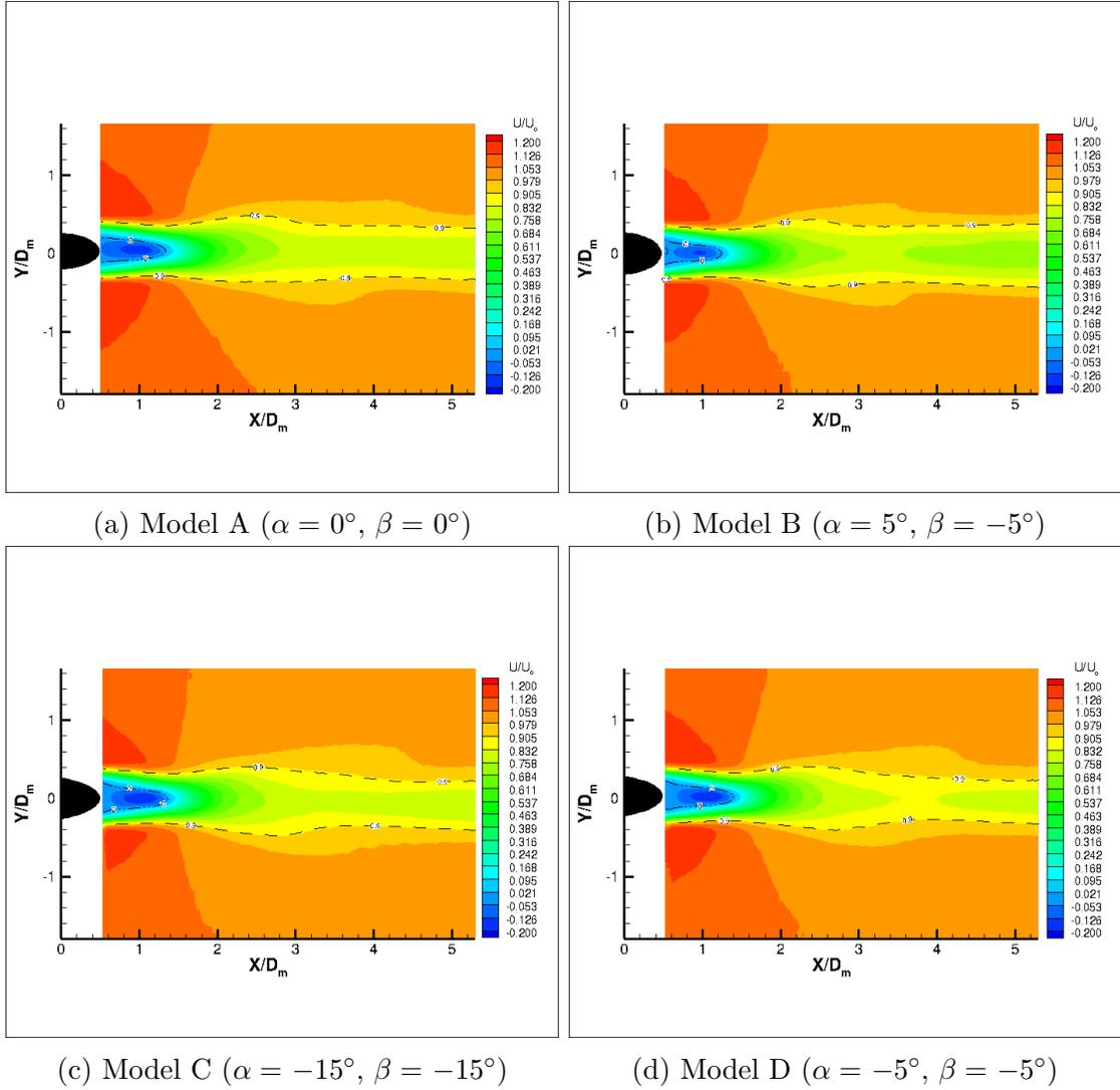
Figure 37: Normalized  $u$  velocity fields in the wake of whisker models A-D (Peak cross section  $x$ - $y$  plane)
