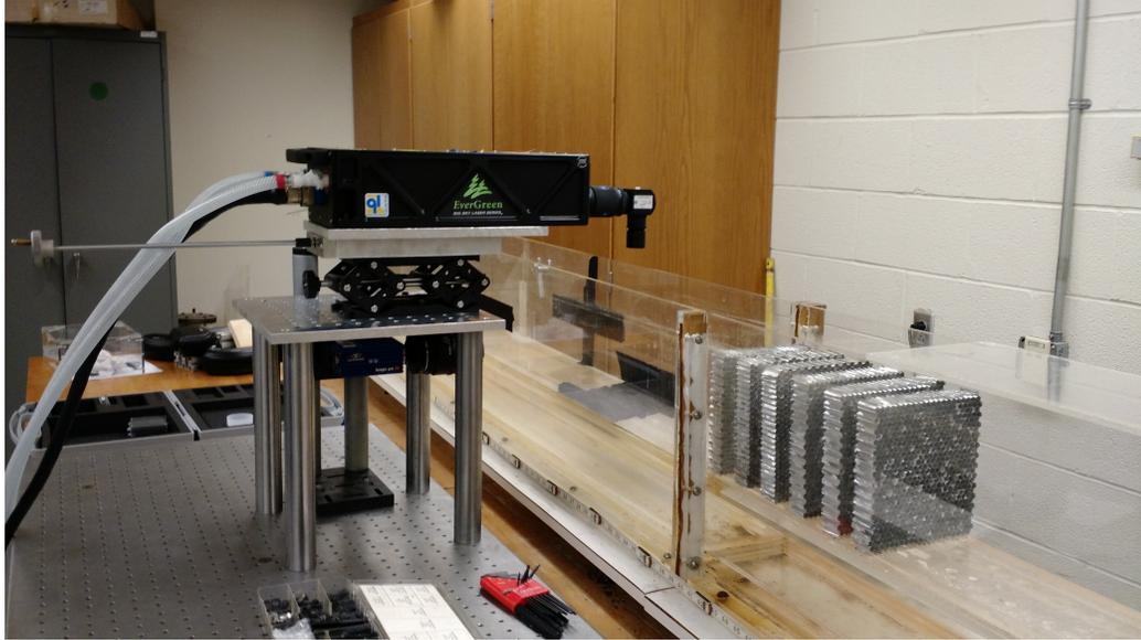
Figure 27: Experimental setup at CSU water channel displaying vertical measurement plane setup: honeycomb flow conditioners, ND:Yag laser, and CCD camera
