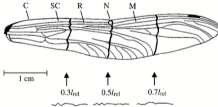
Figure 1: Drawing of dragonfly wing with cross section profiles identifying corrugation [42]
