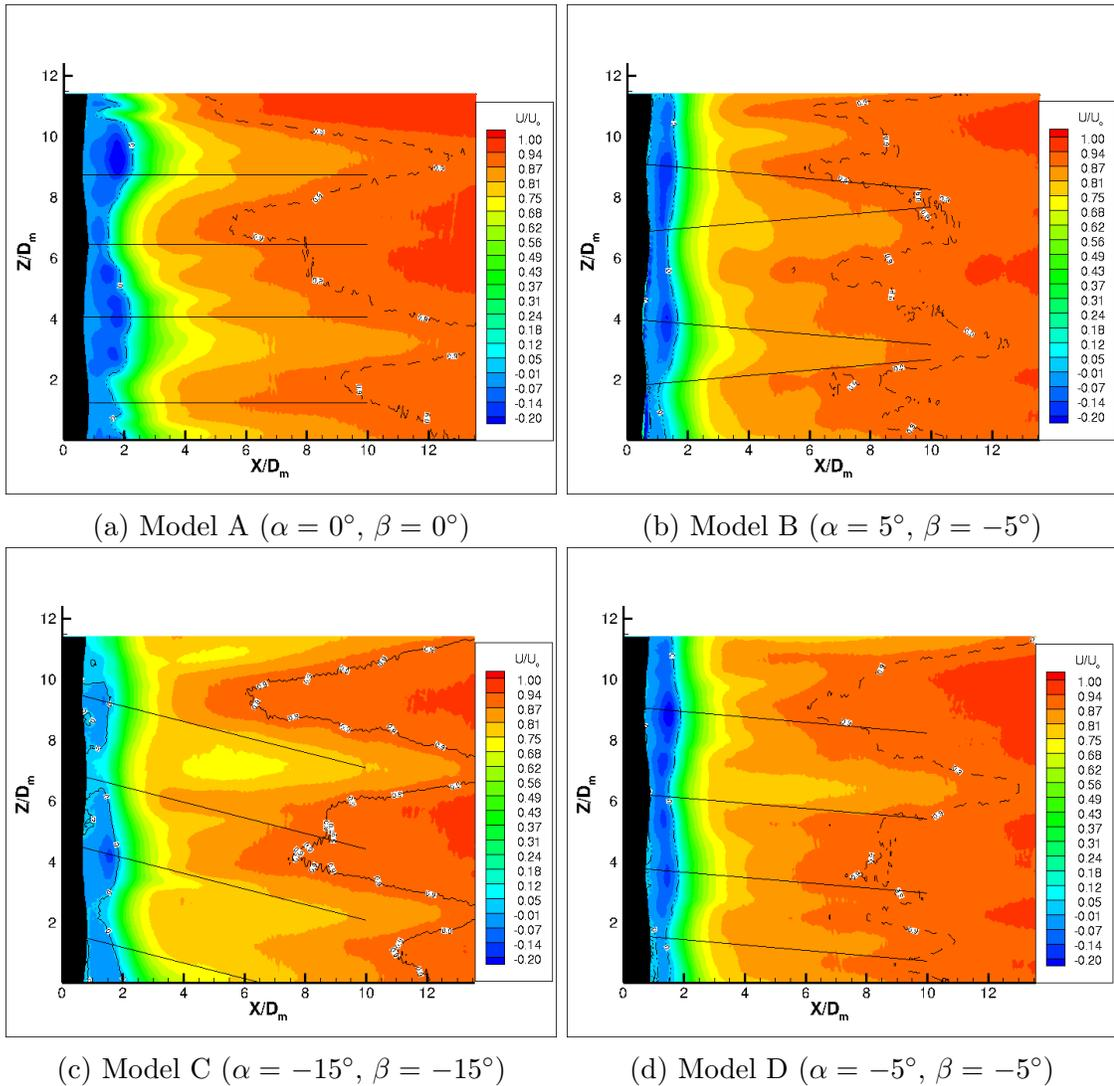
Figure 31: Normalized mean  $u$  velocity fields in the wake of whisker models A-D (Vertical center  $x$ - $z$  plane)
