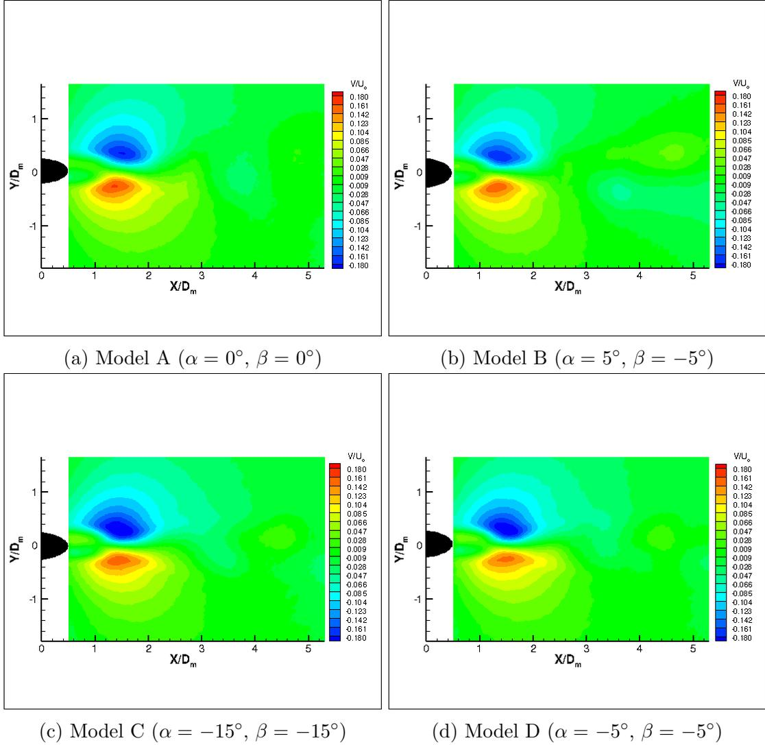
Figure 38: Normalized  $v$  velocity fields in the wake of whisker models A-D (Peak cross section  $x$ - $y$  plane)
