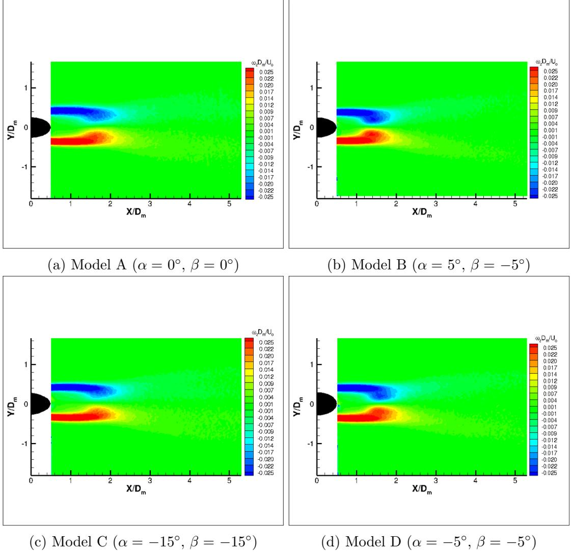
Figure 45: Normalized  $\omega_z$  vorticity fields in the wake of whisker models A-D (Trough cross section  $x$ - $y$  plane)
