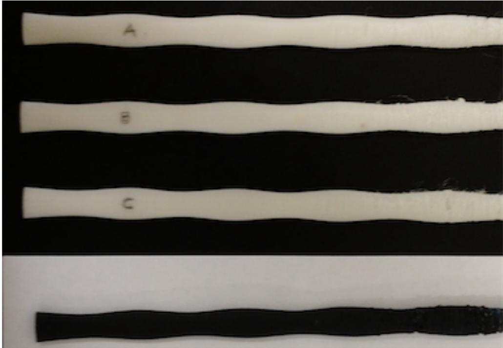
Figure 25: 3D printed whisker models produced with Stratasys uPrintSE Plus 3D printer. Three models shown before application of matte black paint and one after application.
