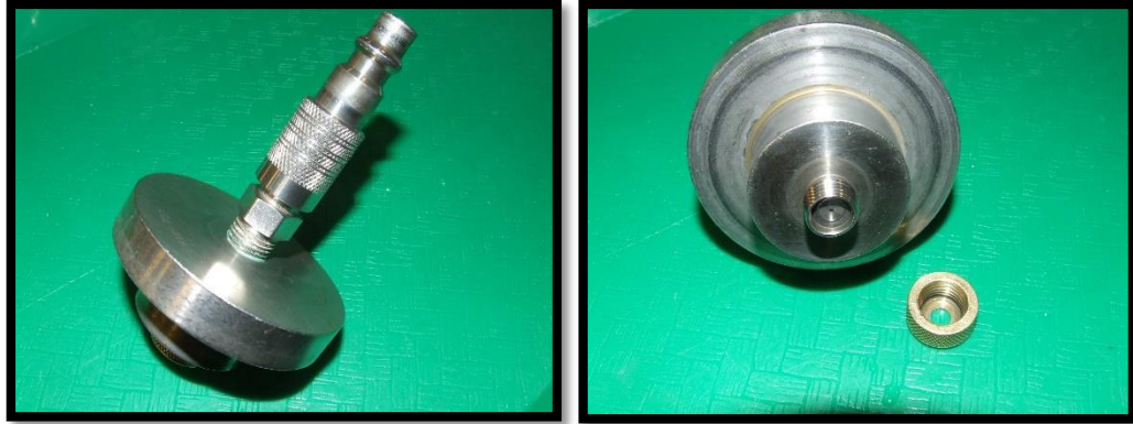
Figure 32: Fixture for Spray Angle Device, Macrospray Atomizer (Source: Parker Hannifin Gas Turbine Fuel Systems Division)
