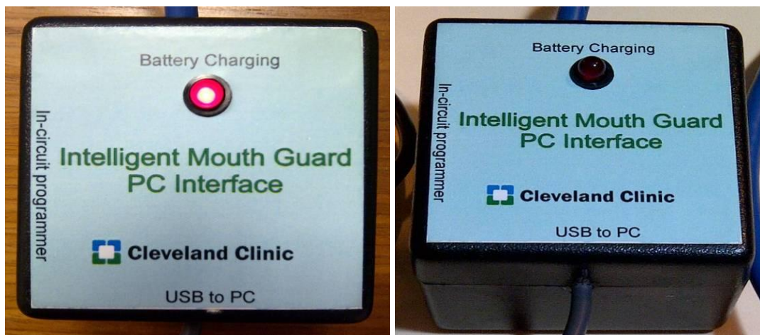
Figure 1.12 LED Located in IMG PC Interface is on ( left ) and off ( right )
