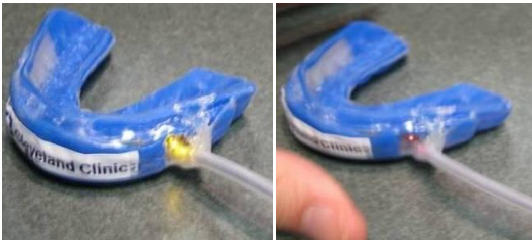
Figure 1.10 IMG LED Blinking Yellow When It Works ( left ) and Blinking Red When It is Triggered ( right ).
