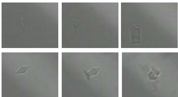
Figure 3.21. Ice crystal morphologies in the presence of the T1N/PAA reaction mixture. c-axis is parallel to the paper plane. Protein concentrations in rows 1 and 2 are 30 and 3 \mu\text{M} , respectively.
