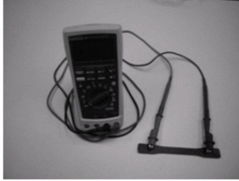
Figure 4.6: Measurement of Resistance using Fluke 189 Multi-meter
