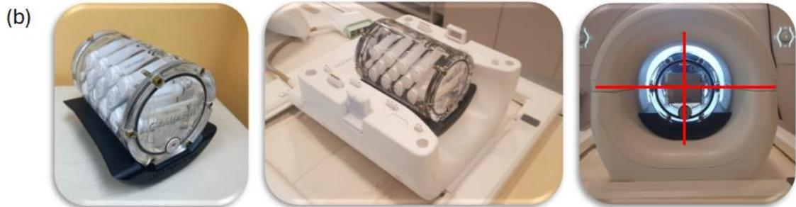
Figure 20 a) Vial position and nominal T<sub>1</sub> and T<sub>2</sub> for each vial. b) Picture of phantom placement on the coil with phantom stand. Phantom stand ensures the phantom is in the middle of the coil consistently.
