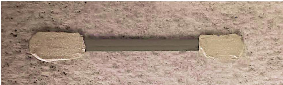
**Figure 3-11:** A 20 mm x 2.5 mm Zn ink sample on a glass slide. The sample was sat on paper for better image capture.
