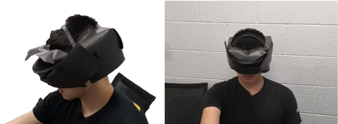
Figure 2.7: Using HoloLens and shroud to simulate VR visualization
