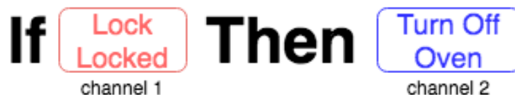
Figure 3.4. An Example of Trigger Action on IFTTT
