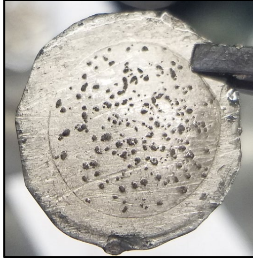
Figure 1.3 - A lithium foil electrode covered with dendrites after Li electrodeposition.
