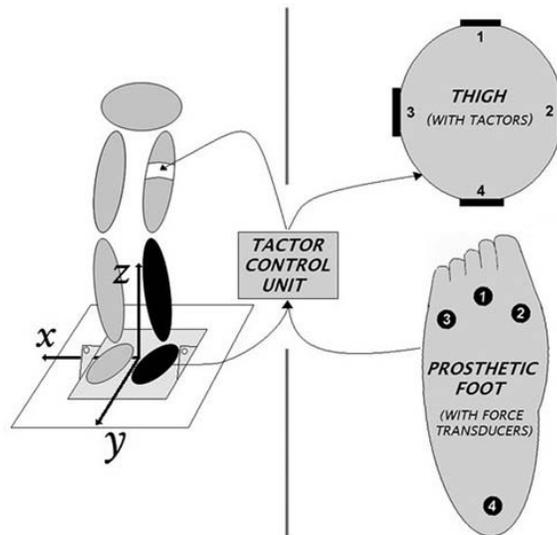
**Figure 5:** Image of below-knee prosthesis with electrocutaneous sensory feedback by Sabolich & Ortega.
