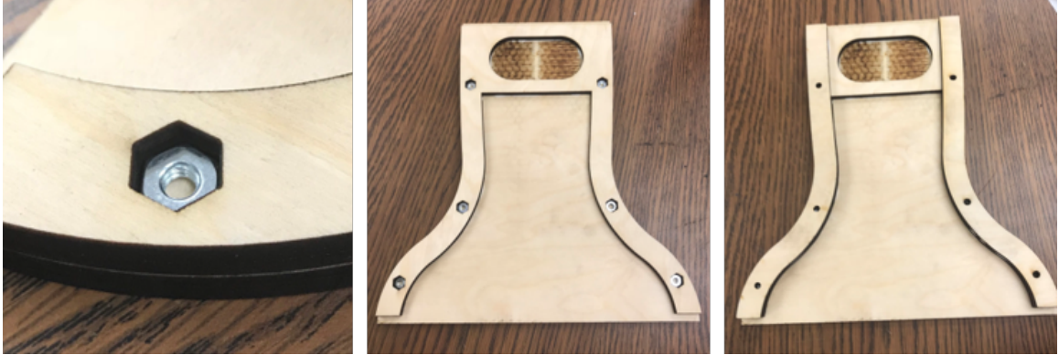
Figure 2.3: Nut assembly images showing closeup of nut in hexagonal hole, six nuts in the torso cover’s second layer, and the torso cover after the third layer is attached.
