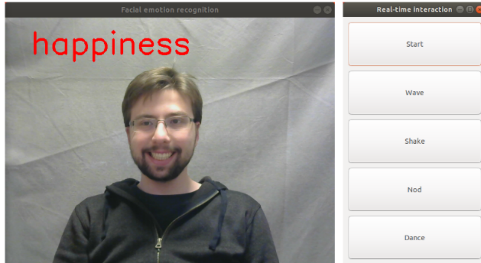
Figure 4.9: Real-time interaction function interface. Left: window shows real-time FER results; Right: window with generated gesture buttons for interaction.
