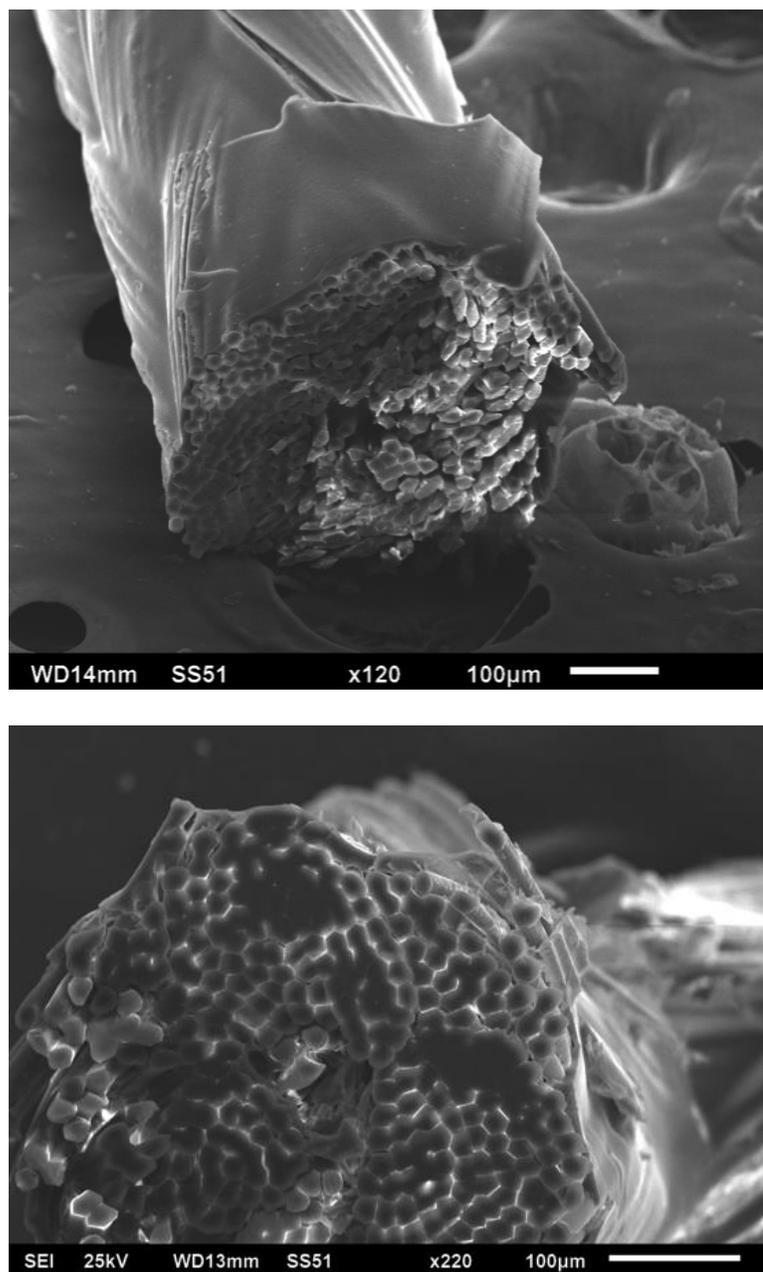
**Figure 2.3.** Scanning Electron Microscopy (SEM) cross-sectional images of non-absorbable nylon sutures with polymerized cyclodextrin (pCD) coating. Scale bar represents 100μm.
