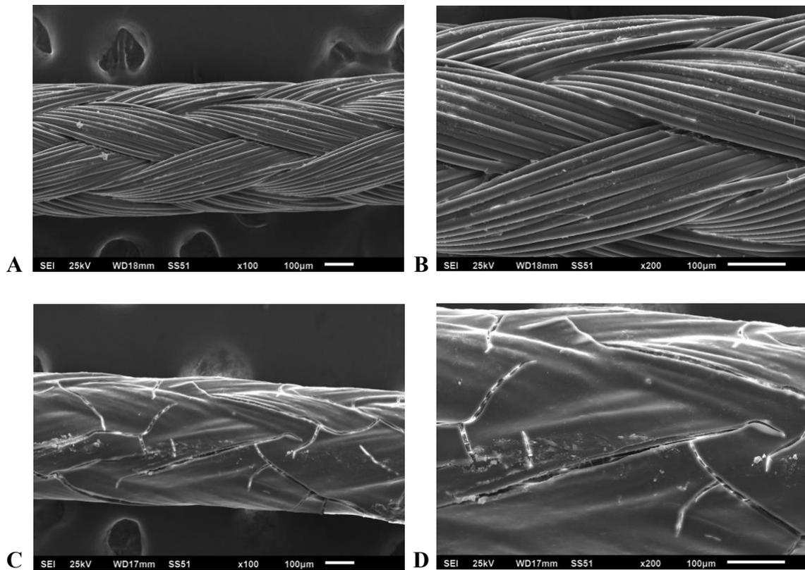
**Figure 2.2.** Scanning Electron Microscopy (SEM) images of non-absorbable nylon sutures before (A, B) and after (C, D) polymerized cyclodextrin (pCD) coating. Scale bar represents 100μm. pCD coated sutures show smoother surface in comparison to individual braided threads which can be seen in the uncoated image, but there is significant micro cracking throughout the coating itself.
