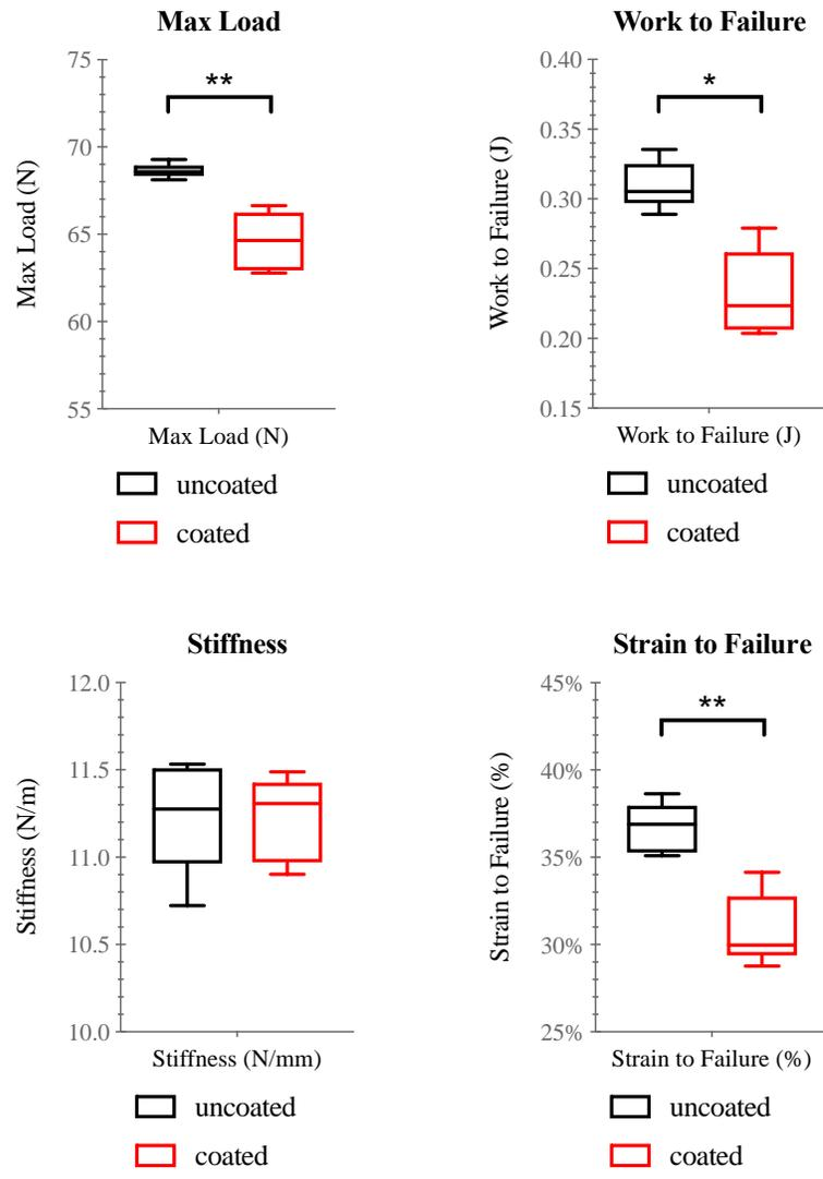
**Figure 2.5.** Tensile testing of polymerized cyclodextrin (pCD) coated and uncoated nylon sutures shows significant difference between Max Load, Work to Failure, and Strain to Failure of the two
