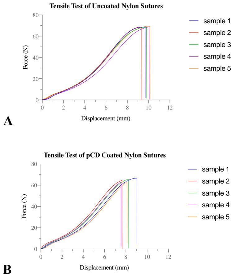
**Figure 2.4.** Force-Displacement curves produced during tensile testing of uncoated (A) and polymerized cyclodextrin (pCD) coated (B) nylon sutures. pCD coated sutures show decreased maximum displacement before failure, and less consistent mechanical behavior.
