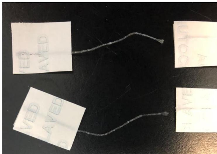
**Figure 3.1** Digital camera images of polymerized cyclodextrin (pCD) coated sutures after undergoing mechanical testing (pull test) and failure. The nylon suture core is black, and the white surface is due to pCD which has partially lifted from the surface.
