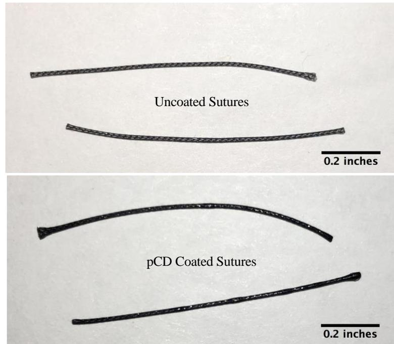
**Figure 2.1.** Digital camera images of non-absorbable nylon sutures with (bottom) and without (top) polymerized cyclodextrin (pCD) coating. Scale bar represents 0.2 in.
