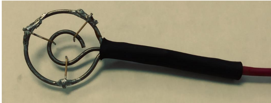
Figure 30: The arrangement of the metal ring and spikes for tests involving several corona showers.
