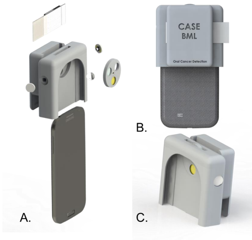
Figure 13: Various views of the FSID. A. Exploded view showing the various components, featuring a rotating filter wheel. B. Front view of the FSID. C. Rear view showing the placement of LED's and filter wheel within the assembly.
