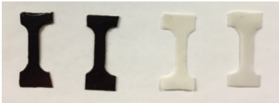
Figure 4.3. PS tensile bars of 10% PS/DNA, 5% PS/DNA, 10% PS/MPP, and 5% PS/MPP from left to right.
