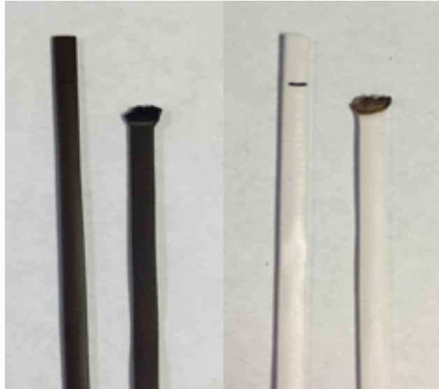
Figure 3.8. LDPE/DNA (left) and LDPE/MPP (right) burn strips before and after burning. Both samples are at a loading level of 30%.
