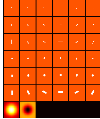
Figure 25: Filter bank designed to capture the calcium characteristics. Each row represents a different scale, where the upper three rows are bar filters in 6 orientations, the three middle rows are edge filters in six orientations and in the last row, Gaussian and Laplacian of Gaussian filters. To generate the MR8 filter responses, only 8 responses are recorded by taking maximal response at each orientation, the Gaussian, and the Laplacian of Gaussian.
