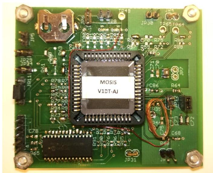
Figure 9-1. WIMM development board used for most wireless recharge tests.
