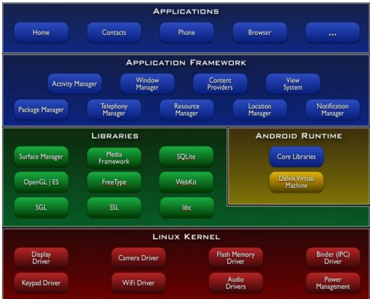
Figure 8: Android operating system architecture
