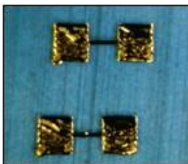
Figure 12 – Partially sintered (10% wt) 500µm long clamp-clamped bridge structures on Corning 0215 soda lime glass.
