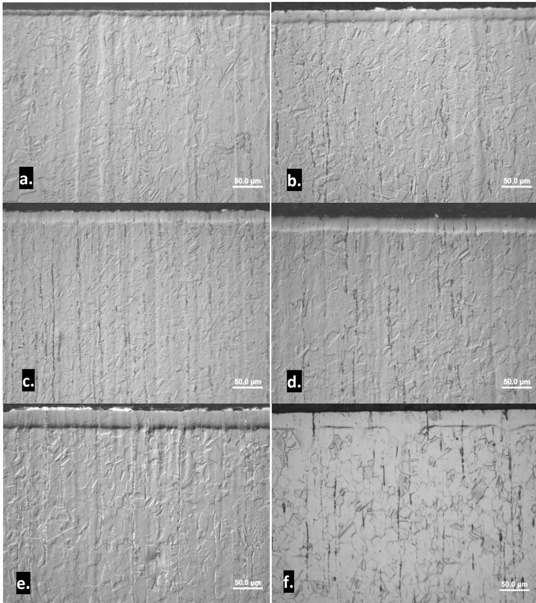
Figure 50 Carburized 316L of varying surface hardness and case depths of (a.) 10 μm, (b.) 15 μm, (c.) 18 μm, (d.) 25 μm, (e.) 30 μm, and (f.) 32 μm
