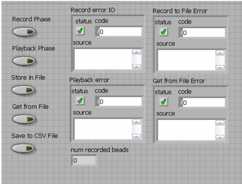
Figure 3-2. The user has five buttons to choose from when teaching and playing back beads. Output errors are also available in the interface.
