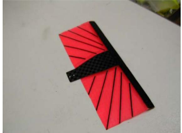
Wing 6: UF Tapered Flexible Wing with 1/8 inch thick LE
