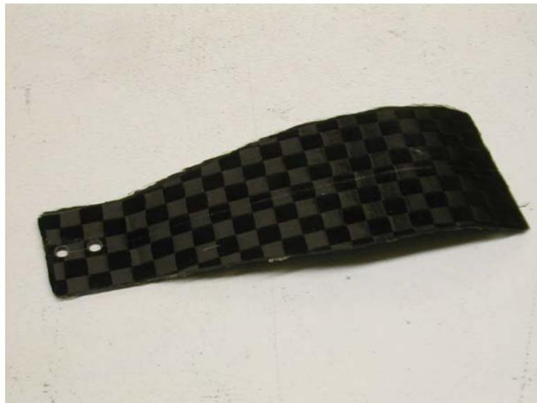
Figure 4.5 – Center wing section used for wing curvature testing
