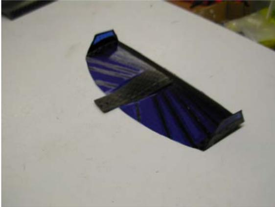
Wing 7: 8300 Rectangular Flexible Wing with 1/8 inch thick LE
