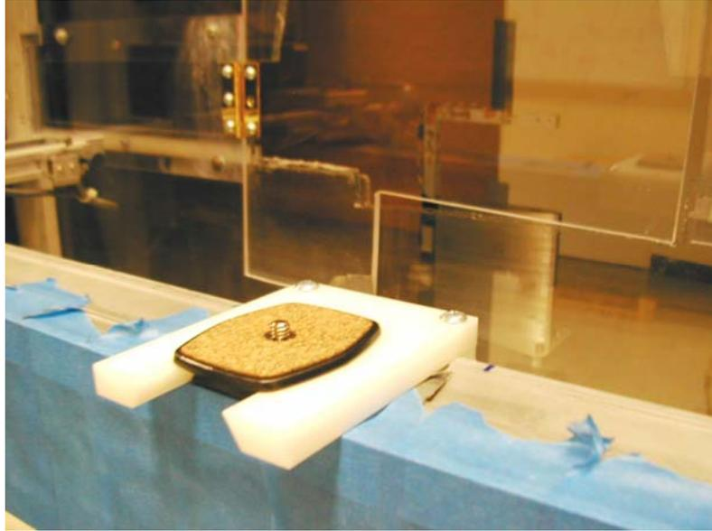
Figure 3.8 – Camera mount attached to wind tunnel side
