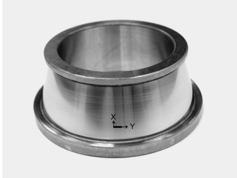
**Figure 2.1.** Approximate location of sample position on cone raceways.
