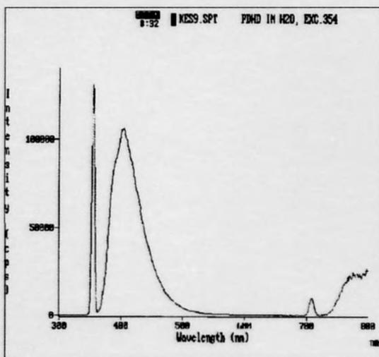
**Figure 16.** Fluorescence spectra of 2.5  $\mu\text{M}$  PDHD, excitation at 354nm.
