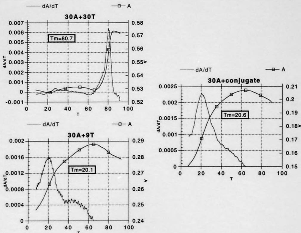
**Figure 18.** Melting curves. A vs. T and calculated  $dA/dT$  vs. T of 30A+30T, 30A+9T and 30A+conjugate in 10mM sodium phosphate, 1M NaCl, pH 7.4.
