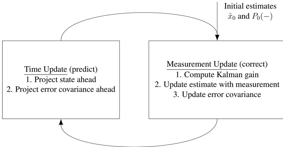
Figure 2.3 Kalman Filter flow diagram.
