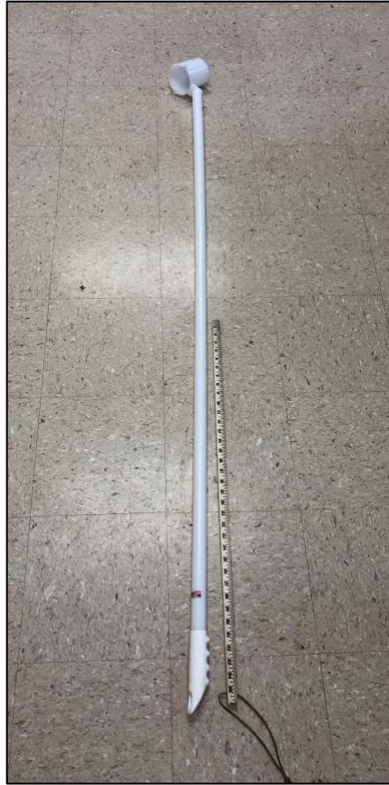
Figure D3. Shows the long-arm sample dipper used to collect grab samples from the surface of combined sewer overflow outfalls. A 36-inch measuring stick is incorporated into the picture for reference.
