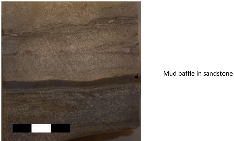
Figure 47. Mud baffle in quartz arenite acting as a barrier to fluid flow. Scale bar = 3 cm.
