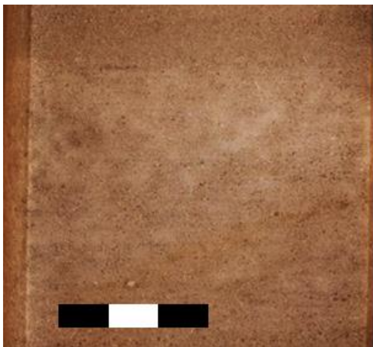
Figure 22. Massive mottled sandstone (lithofacies Smm) from core # 2989. Scale bar = 3 cm.
