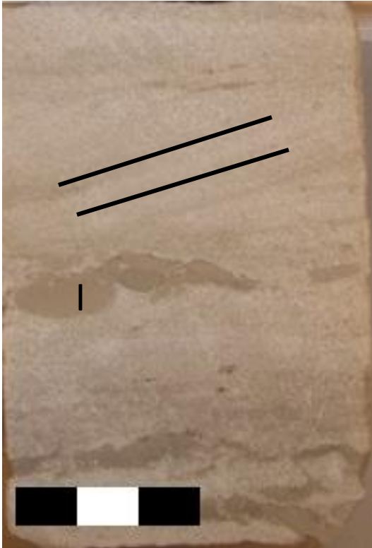
Figure 24. Massive sandstone with intraclasts (lithofacies S mi ) and planar-tabular cross bedded (lithofacies S p ) from core # 2923. Scale bar = 3 cm. I = Intraclast
