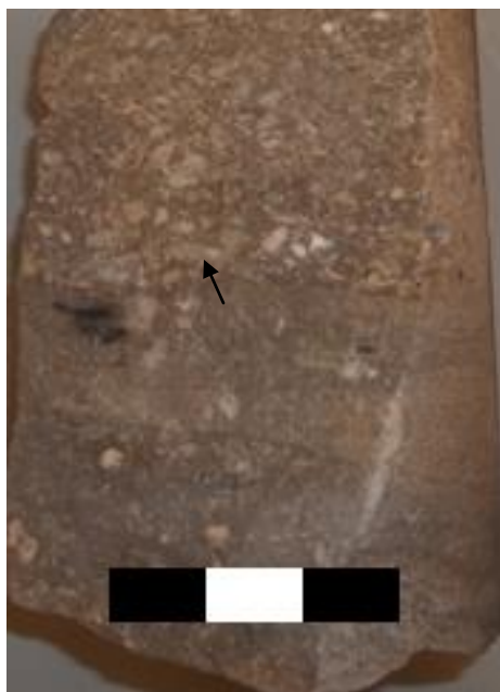
Figure 29. Dolo-packstone with rip up clasts (shown by arrow) in core # 2923. Scale bar = 3 cm.
