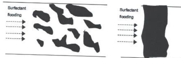
**Figure 3.3.** Surfactant flooding through a cavity with filled with oil.<sup>2</sup>
