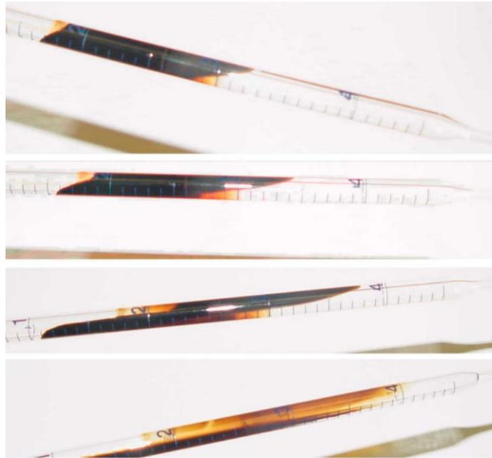
**Figure 3.7.** Pipette from a microemulsion phase behavior salinity scan experiment being inverted.<sup>7</sup>
